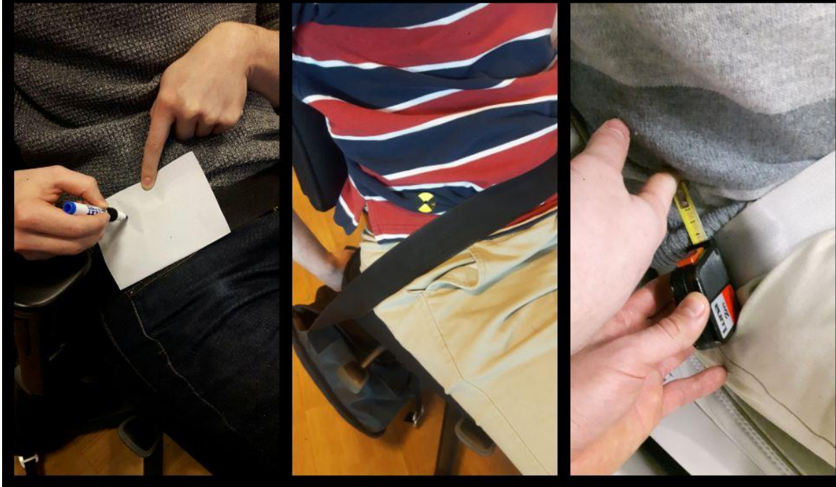
Figure 3.14 - Picture illustrating the three ideas on how to measure the ASIS location in relation to the seat belt. Folded paper, sticker and pointing finger.
