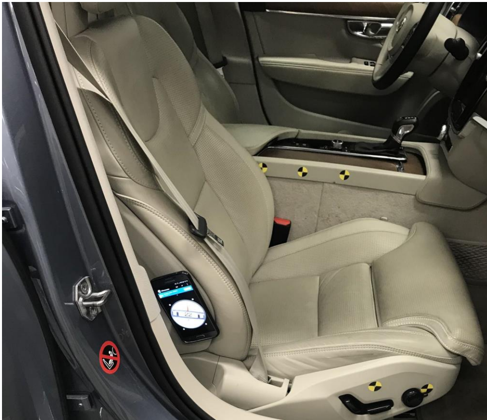
Figure 3.12 - Picture showing how the backrest angle was measured. (The smartphone was attached to the seat using Velcro tape).
