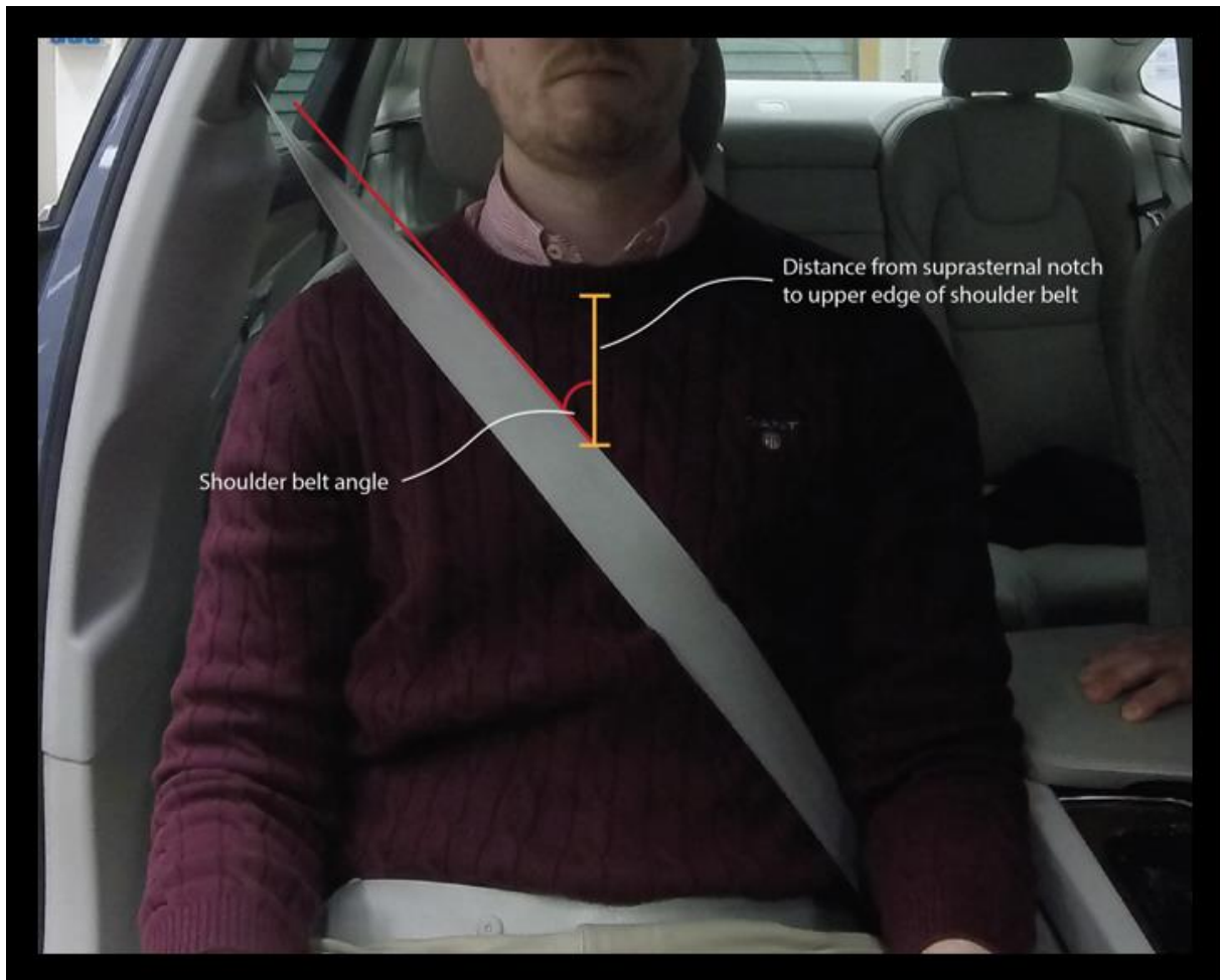
Figure 3.5 - Visualization of how the shoulder belt angle and distance between the suprasternal notch and the upper edge of the seat belt was measured.
