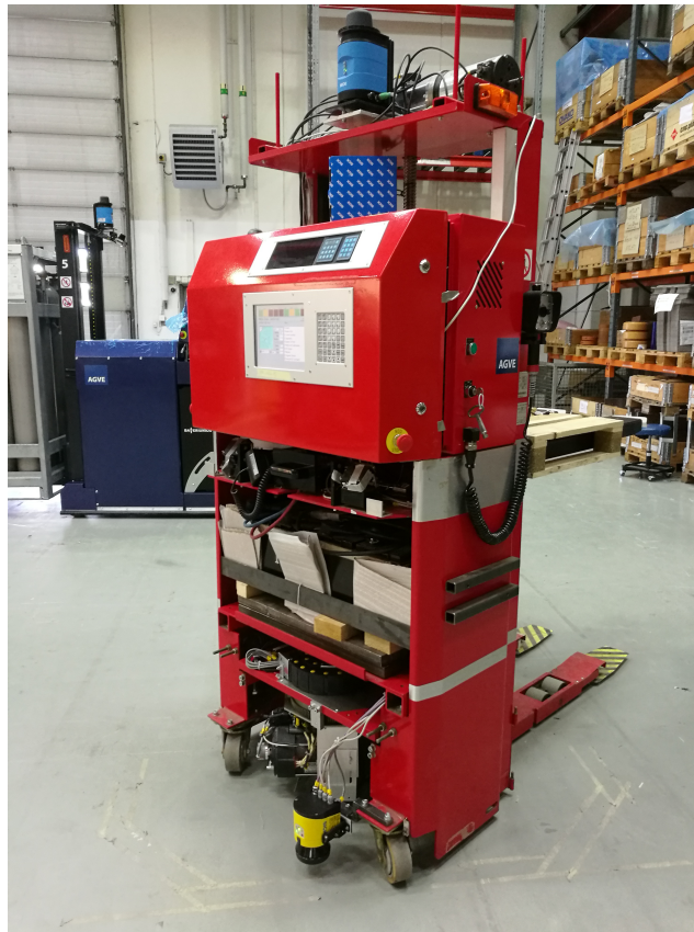
Figure 1.1: A tricycle AGV on which the implementation has been made, at AGVE
