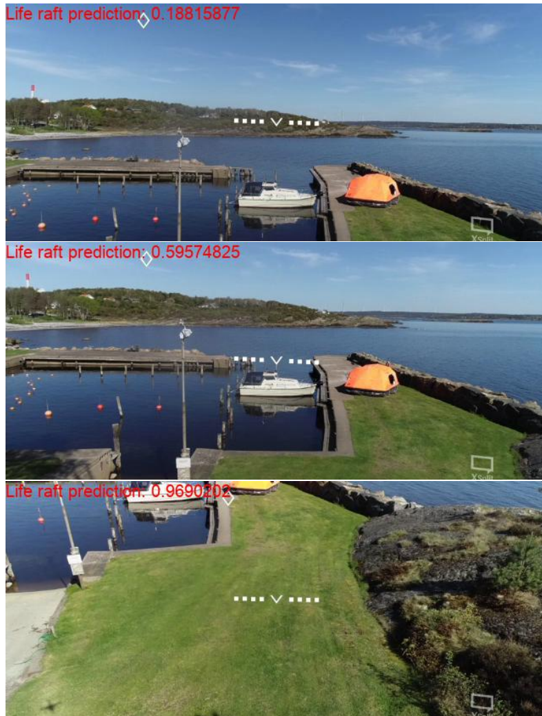
Figure 32: Image series of three consecutive liferaft images displaying the liferaft prediction result in each image with changed training parameters and added images, 18.81% in the top image, 59.57% in the middle image, and 96.90% in the bottom image.
