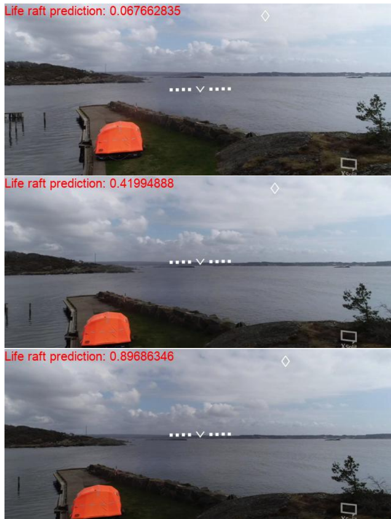
Figure 31: Image series of three consecutive liferaft images displaying the liferaft prediction result in each image, 6.77% in the top image, 41.99% in the middle image, and 89.69% in the bottom image.
