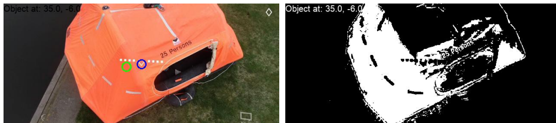
Figure 14: Representation of the color search algorithm, the upper image illustrates the distance calculation. The green circle represents the center of the detected object, the blue circle illustrates the center of the image. In the top left corner of the upper image, the distance of the object relative to the image center is display, 35 pixels in x-direction and -6.0 pixels in the y-direction. The lower image is the grey-scale image with the red/orange areas highlighted.
