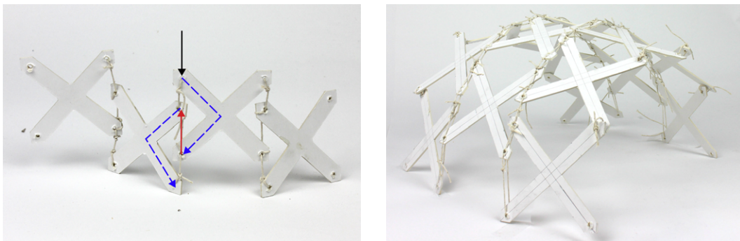
Figure 3.6: Tensegrity system using compression crosses and tension cables
