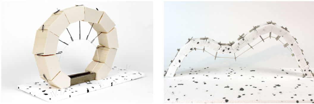
Figure 3.7: Funicular shapes altered with external prestressing
