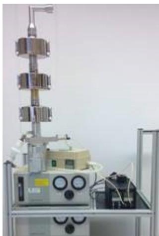
Figure 3.13: *View of the experimental testing instrumentation. In the left upper corner, the USP throat to which the devices were attached can be seen. The USP throat is connected underneath to three pre-separators, as was used for the testings on the  $\Omega$ -bend devices. The pre-separators are in turn connected to the APS, that can be seen in the lower part of the figure.*
