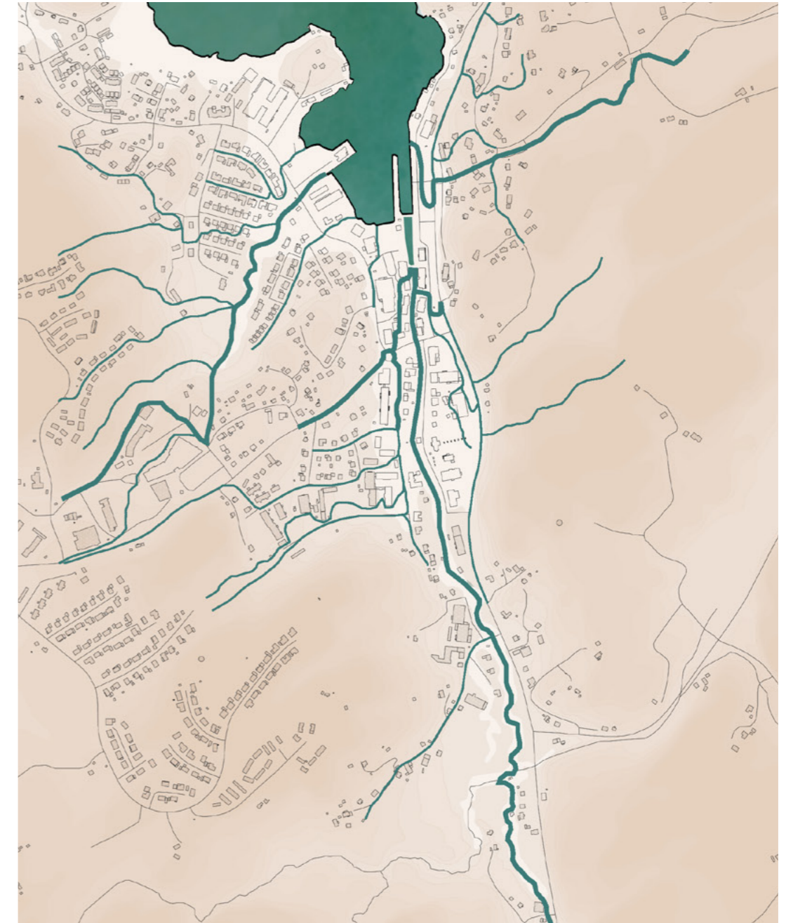
Figure 7.2. Main waterflows in case of heavy rains
