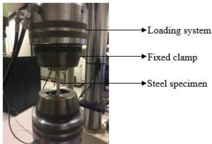
Figure 3.7: Performed tensile test on specimen (MTS machine).
