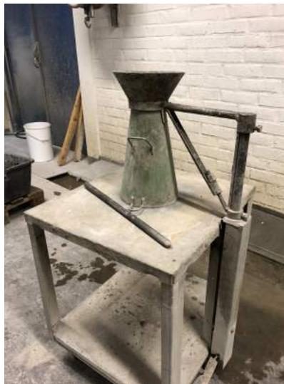
Figure 6.6 Arrangement for slump test.
