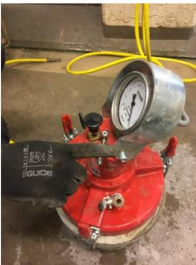
Figure 6.7 Gauge pressure meter used for determining of air content.
