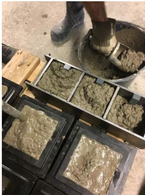
*Figure A.1 The two different test-cubes with the internal vibrator.*
