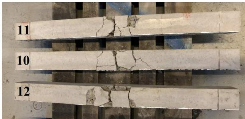
Figure C.8 Beam 10-12 looking at the bottom of the beam.
