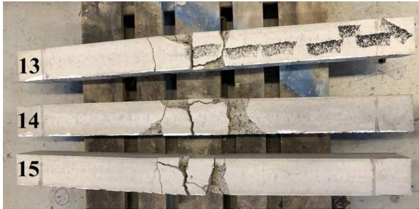
Figure C.6 Beam 13-15 looking at the bottom of the beam.
