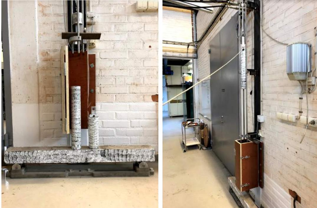
(a) Placing of the beam. On top of the beam is the two drop-weights.
