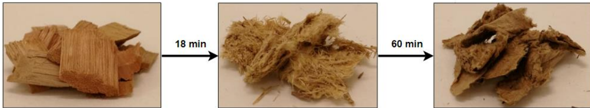
Figure 24. The path from wood chip to pulp during the L cook. First 18 min cook and then 60 min. The 22,6 min cook is not included since there are no visual difference between that and the pulp cooked for 18 minutes.
