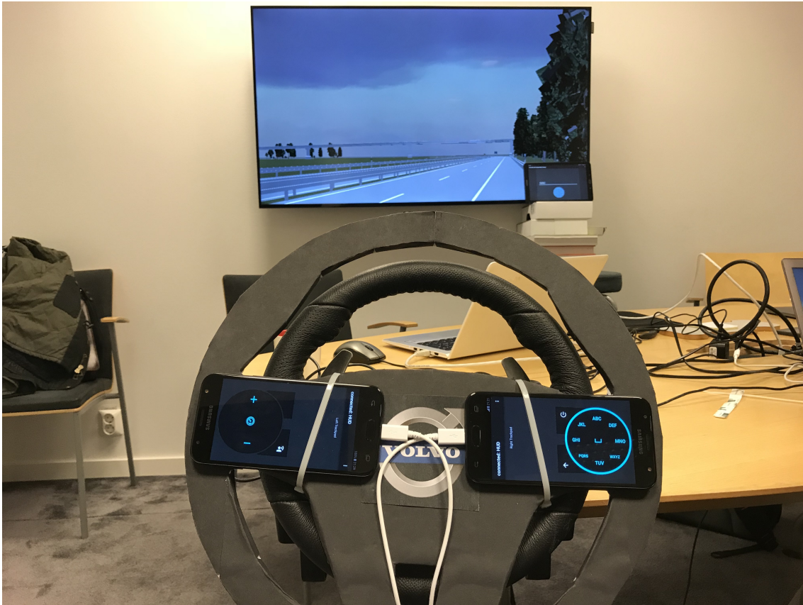
Figure 5.23: The steering wheel prototype used for the second and third user test. Symbols: [12, 22, 23, 33, 34, 35, 54].
