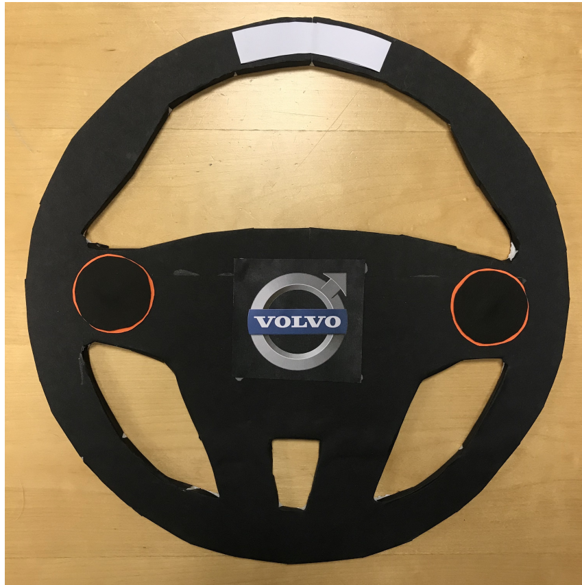
Figure 5.10: The tangible prototype of a steering wheel with the trackpads. Symbols: [54].
