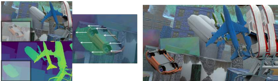
(a) Left image and right disparity map together with how the pixels are selected when warping the image (b) Warped right image I'_r
