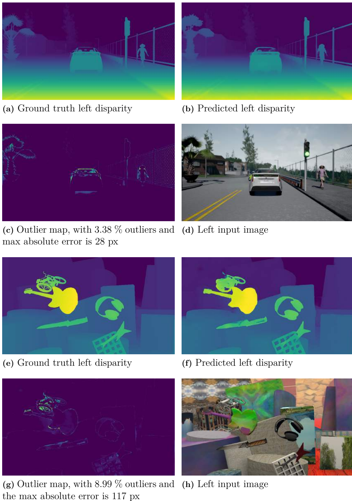
Figure 3.12: Results from the X-CNN network trained on Carla, image (a)-(d), and FT3D, image (e)-(h), respectively. The network does not perform well on edges and occluded areas. The outlier map is a heat map for all the pixels labeled as outliers.
