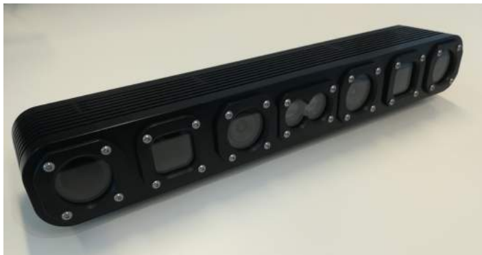
Figure 3.1: The camera rig consisting of four cameras and a laser rangefinder.
