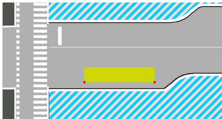
**Figure 3.13:** Red dots: Placement of Lidars on the bus for detection of persons in concept solution during docking.
