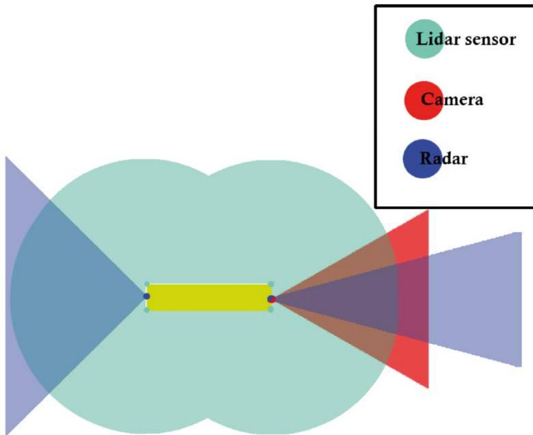
**Figure 3.15:** Concept 2: Lidar-based SLAM with extended sensor suite.
