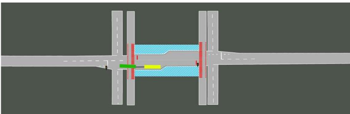
**Figure 3.10:** Docking-phase start (green) and stop (yellow) position of autonomous vehicle.
