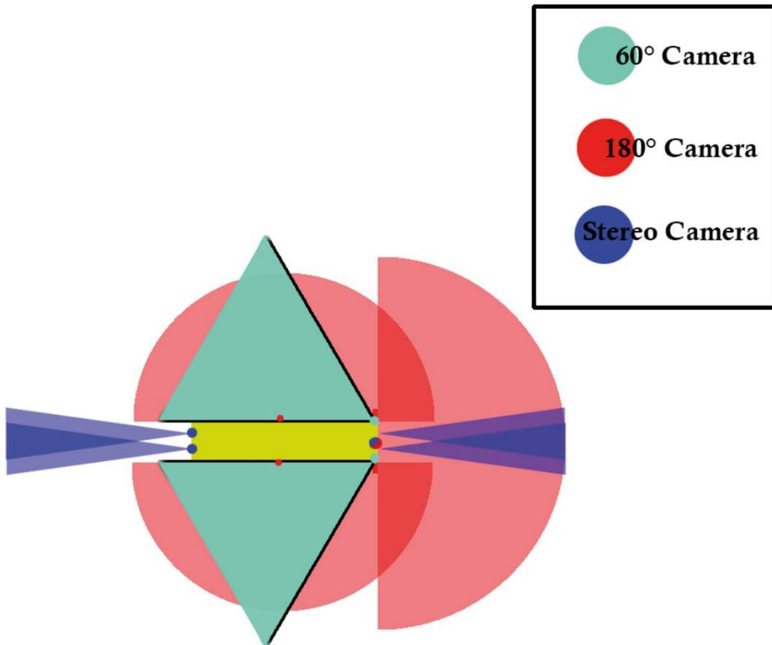
**Figure 3.16:** Concept 3: Sensor suite consisting of only cameras.
