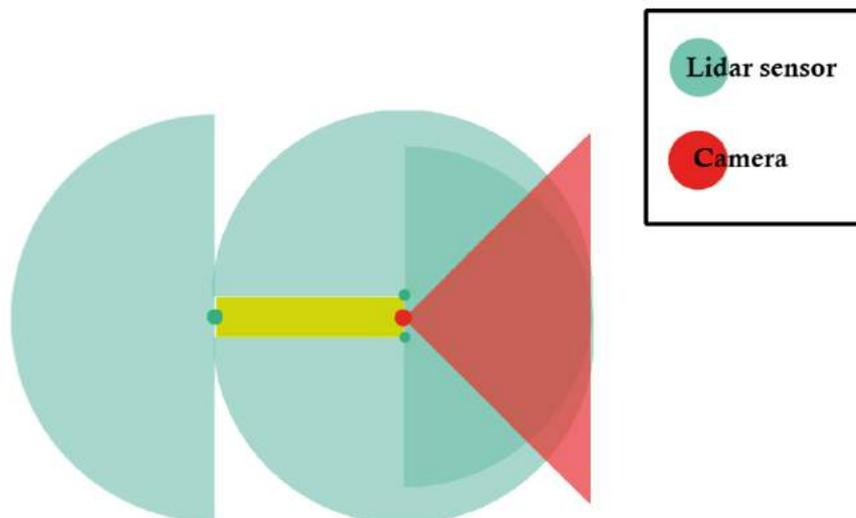
**Figure 3.14:** Concept 1: Lidar-based SLAM with an optical sensor.
