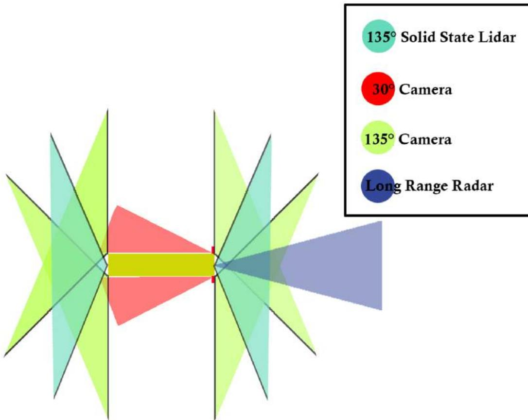
**Figure 3.17:** Concept 4: Sensor placement overview
