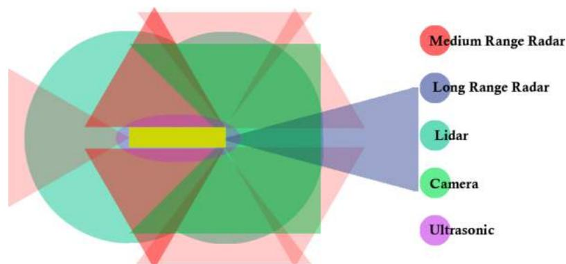
**Figure 4.3:** Total sensor coverage of final concept.
