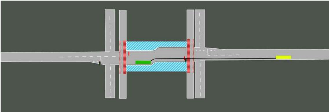
**Figure 3.12:** Departure-phase start (green) and stop (yellow) position of autonomous vehicle.
