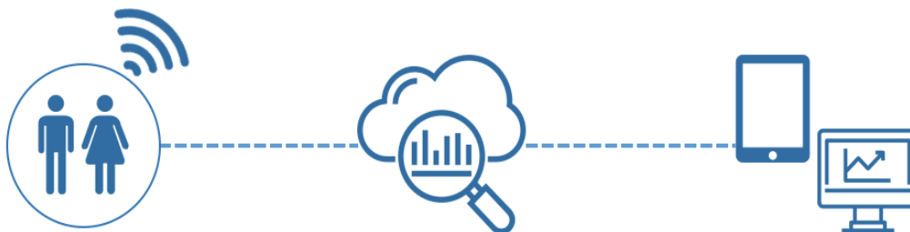
Figure 10. An illustration of the Tork EasyCube and its three main modules; (1) the sensor technology that measures the number of visitors, levels of refill and the transmits data, (2) the data is collected and aggregated on Essity's servers and (3) that customer access the data through the Tork EasyCube web application.
