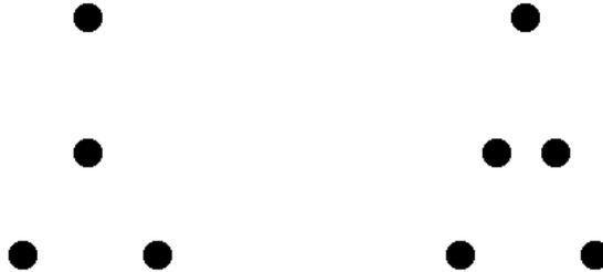
**Figure 3.4:** IR LED arrangement for car 0 (left) and car 1 (right)
