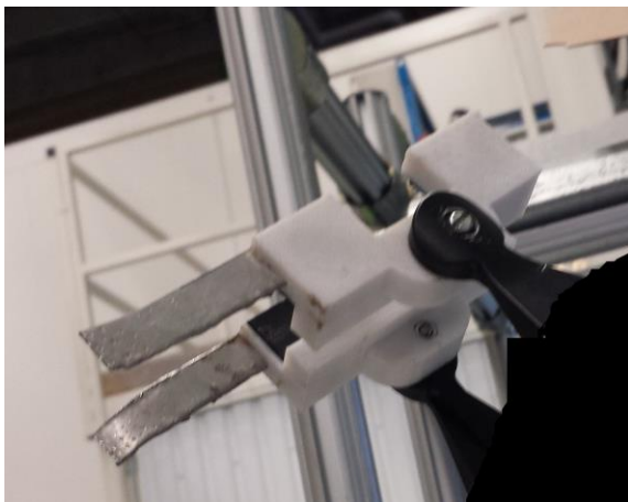
Figure 8. The final version of the fingers, mounted on the robot's gripper
