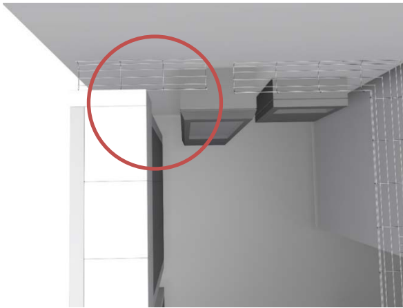
Figure 9.1. Issue with switchboard and cooling units being close to each other.
