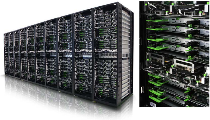
Figure 2.5. OCP Open Rack V2 with OCP IT hardware (Shi, 2014)
