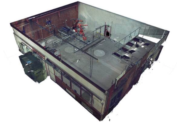
Figure 5.2: An example of a 3D laser scanned production environment from Chalmers Production System Laboratory.
