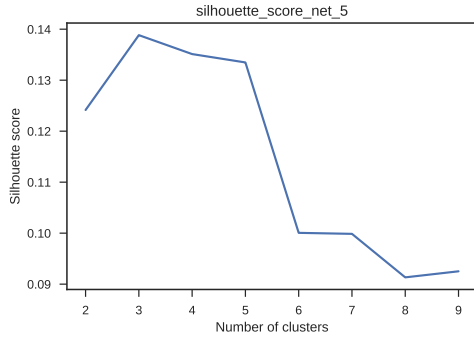
Figure 4.10: The silhouette score for different values of k in the k-means clustering algorithm when clustering on the latent subspace of net 5 .
