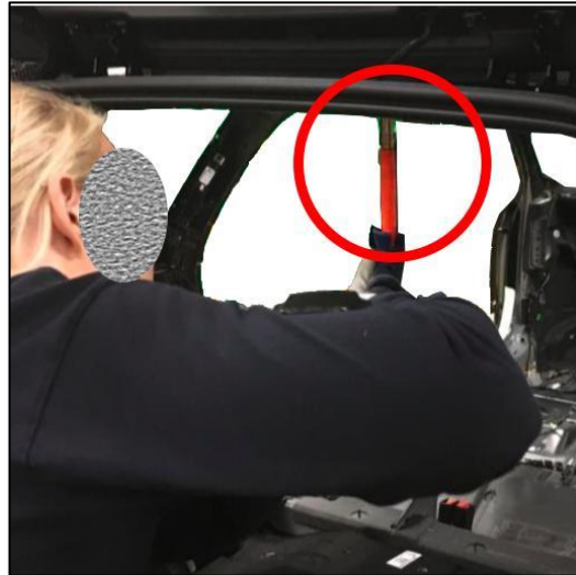
Figure 25 - Fastening of antenna amplifier with a heavy screwdriver in an awkward posture and in red zone. Photo used with permission from Volvo Car Corporation.
