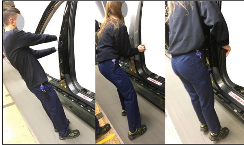
Figure 31 - Fastening of upper (left picture) and lower (middle and right picture) B-panel. Photo used with permission from Volvo Car Corporation
