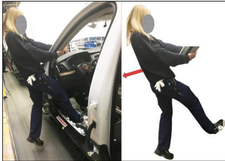
Figure 30 - Fastening of A-panel by swinging the body backwards. Photo used with permission from Volvo Car Corporation
