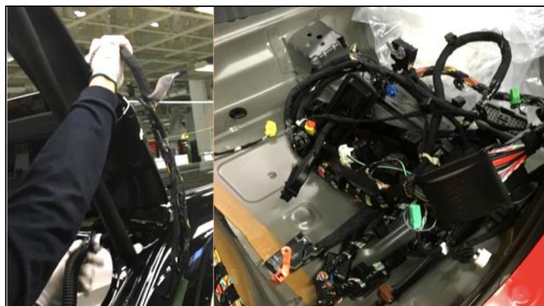
Figure 24 - To the right; A tailgate harness is being entered in a narrow hole, carried out in a red working zone, too high up. To the right; a floor harness placed in the middle of the car floor before assembly is carried out. Photo used with permission from Volvo Car Corporation.
