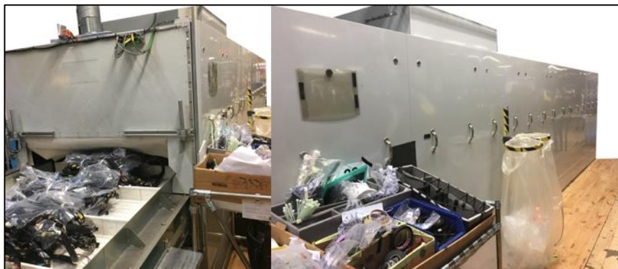
Figure 33 - Oven used for heating of wire harness. Photo used with permission from Volvo Car Corporation
