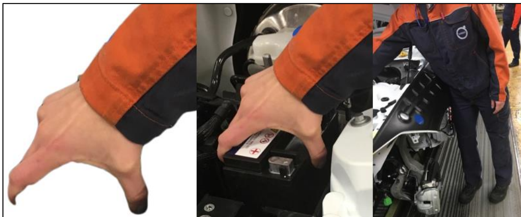
Figure 27 - Positioning of the battery with hook grip, abducted arm and bent back. Photo used with permission from Volvo Car Corporation
