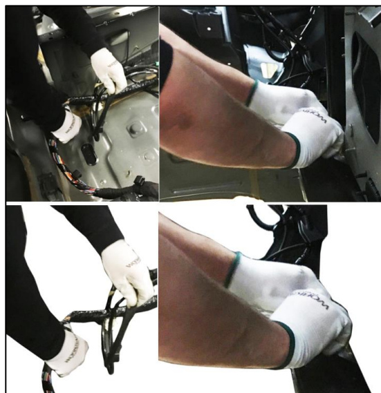
Figure 32 - Fastening of wire harness in the floor and the engine bay. Photo used with permission from Volvo Car Corporation
