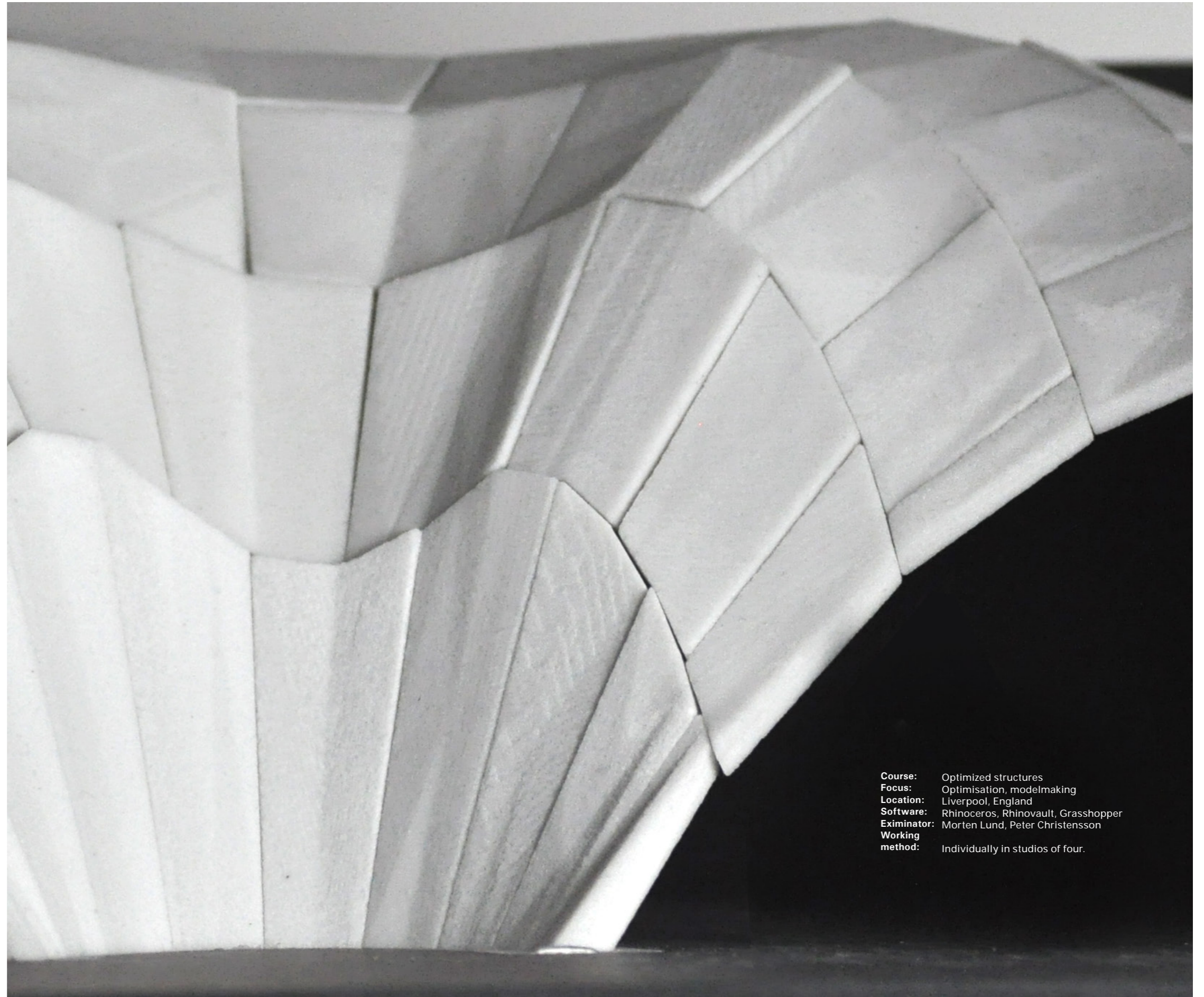
No glue needed Close-up of the self-bearing shell structure. Mdf, hardened gypsum, 1:50
