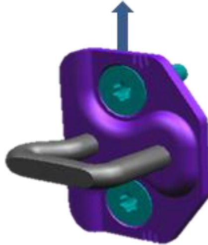
Figure 7. The adjustment of X_2 Striker Alignment. The arrow shows the direction of the adjustment.
