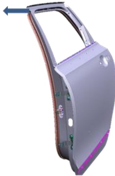
Figure 8. The adjustment of X 3 door frame. The arrow shows the direction of the adjustment.
