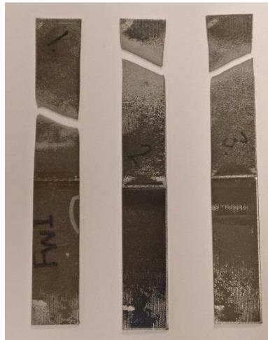
Figure 68. FW (FW & No ablation), sample 1 to 3 after tensile testing
