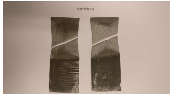
Figure 62. FW (FW & No Ablation) X, sample 1 & 2 after tensile testing
