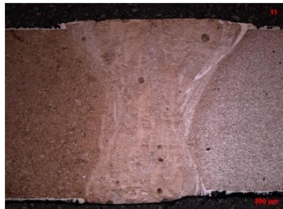
Figure 52. Macrograph of the FW-welding process (FW & No ablation)
