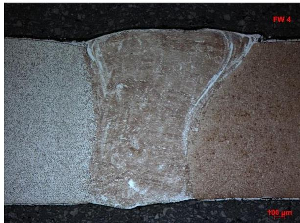
Figure 54. Macrograph of the FW-welding process (FW & No ablation)
