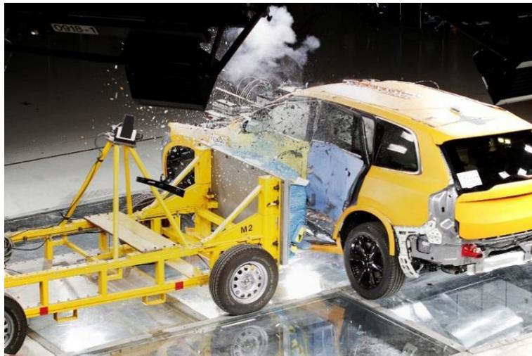
Figure 2. Side collision [1]
