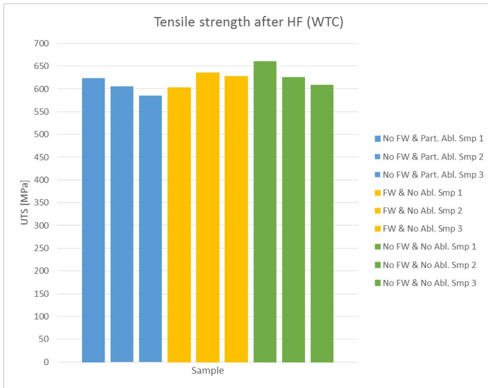
Figure 70. Bar chart showing Tensile strength for weld test coupon samples
