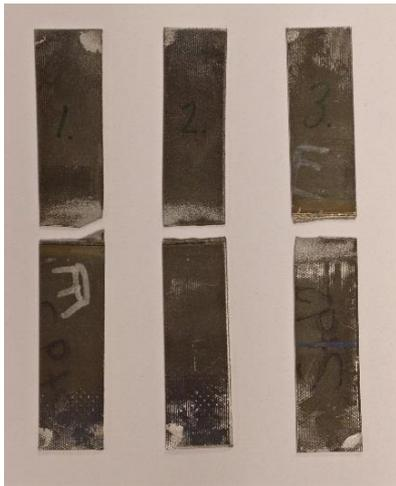
Figure 67. STD (No FW & Partial ablation), sample 1 to 3 after tensile testing
