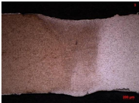
Figure 51. Macrograph of the STD-welding process (No FW & Partial ablation)
