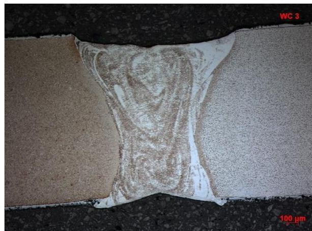
Figure 55. Macrograph of the WC-welding process (No FW & No ablation)
