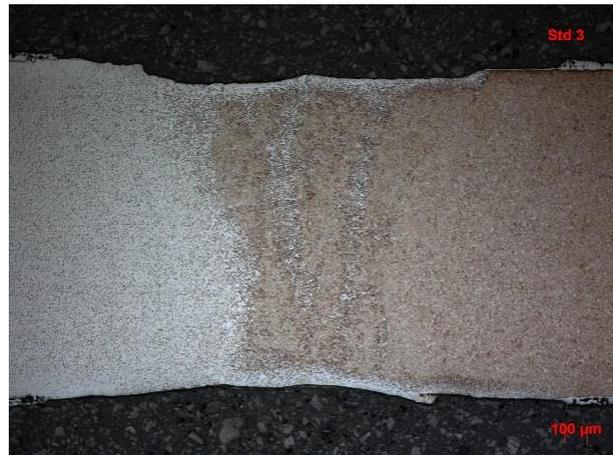
Figure 53. Macrograph of the STD-welding process (No FW & Partial ablation)
