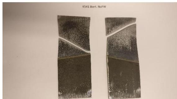
Figure 63. STD2 (No FW & Partial Ablation) Y, sample 1 & 2 after tensile testing
