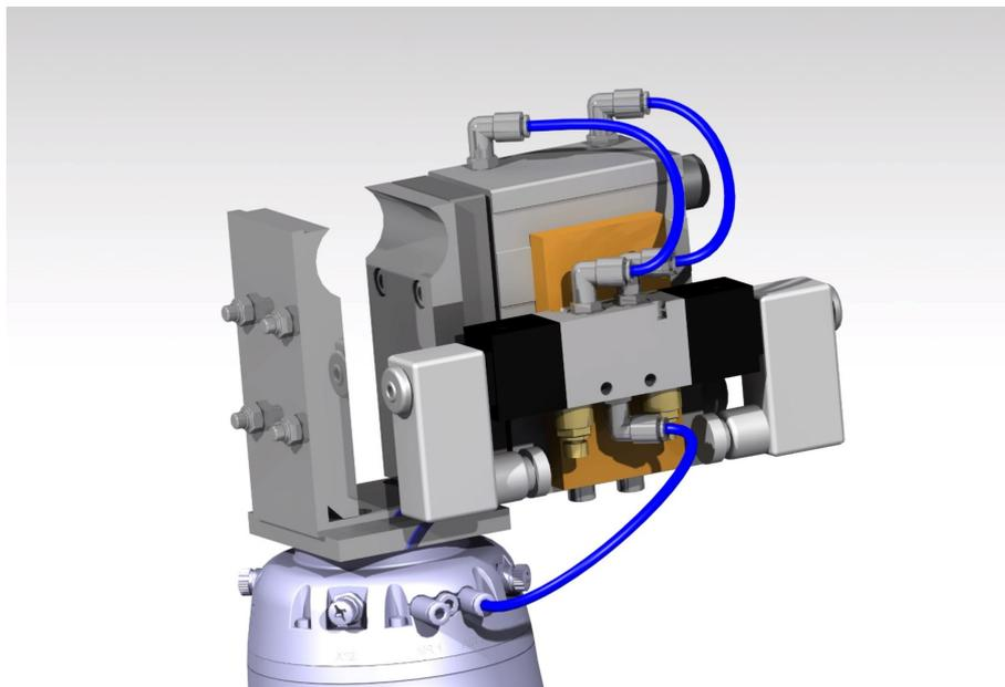
**Figure 4.7:** 3D-model of the gripper mounted to the robot.
