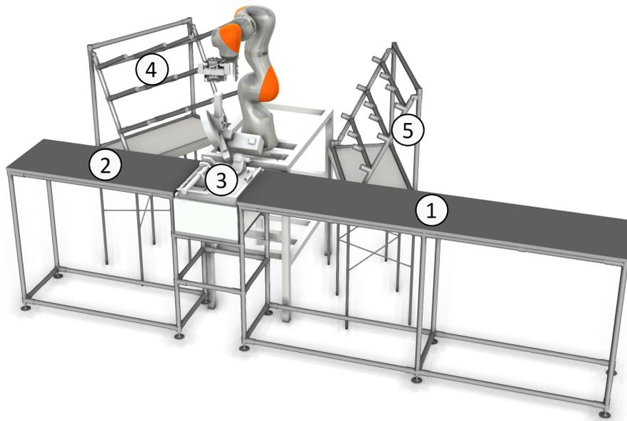
**Figure 4.8:** Layout including robot, mount, gripper, workbench, cutting machine, kitting rack, and buffer rack.
