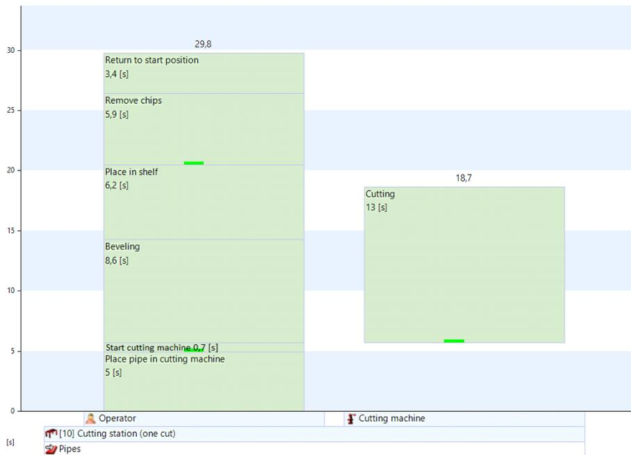
**Figure 4.2:** Time consumption for operator and machine in the current state in a snap-shot from AviX.
