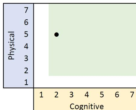
**Figure 4.6:** Analyzed LoA in the current state. The dot represents the current LoA and the green area marks the minimum and maximum LoA of the station.
