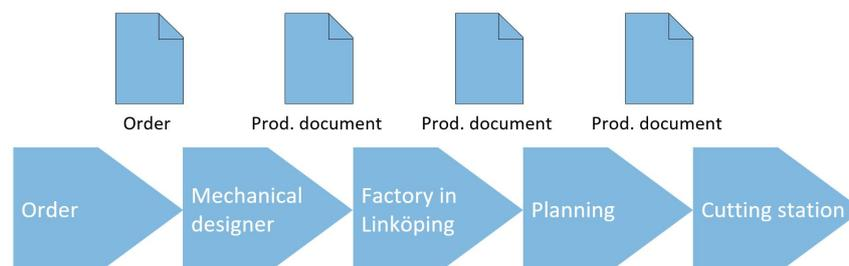
**Figure 4.4:** The flow of information from the order being placed until the operator in the cutting station receives the cutting instructions.
