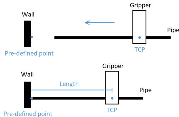
**Figure 3.2:** A visualization of the measuring process in the experiment.
