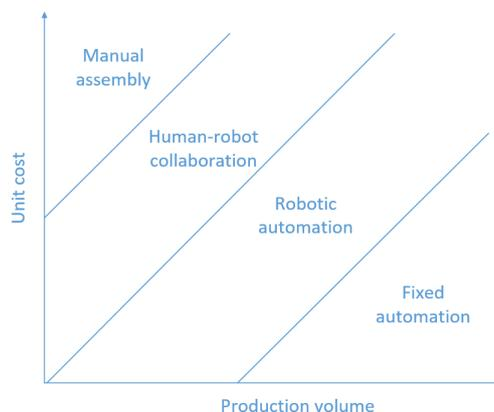
**Figure 2.1:** Level of automation with respect to unit cost and production volume.
