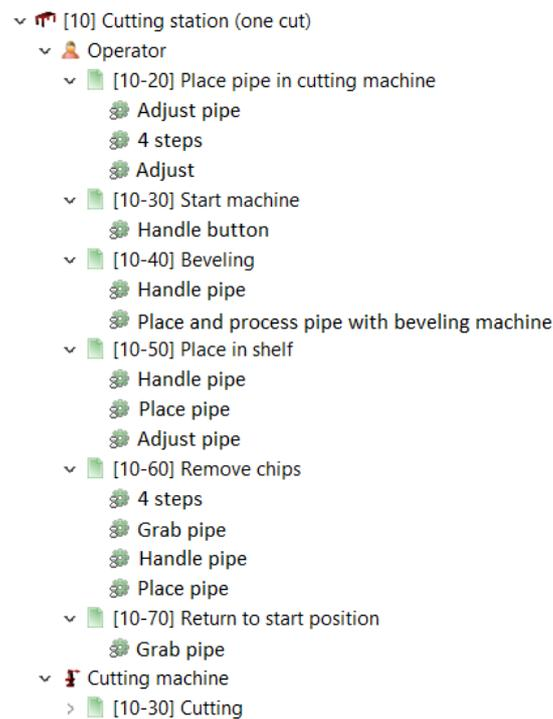
**Figure 4.3:** Task-breakdown of the cutting process made in AviX.
