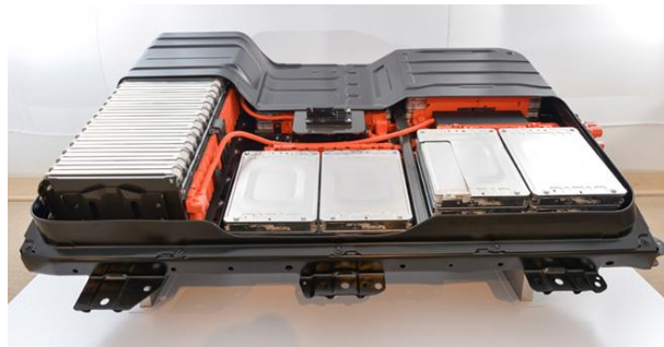
Figure 18. Lithium-ion battery pack (Morris, 2018).
