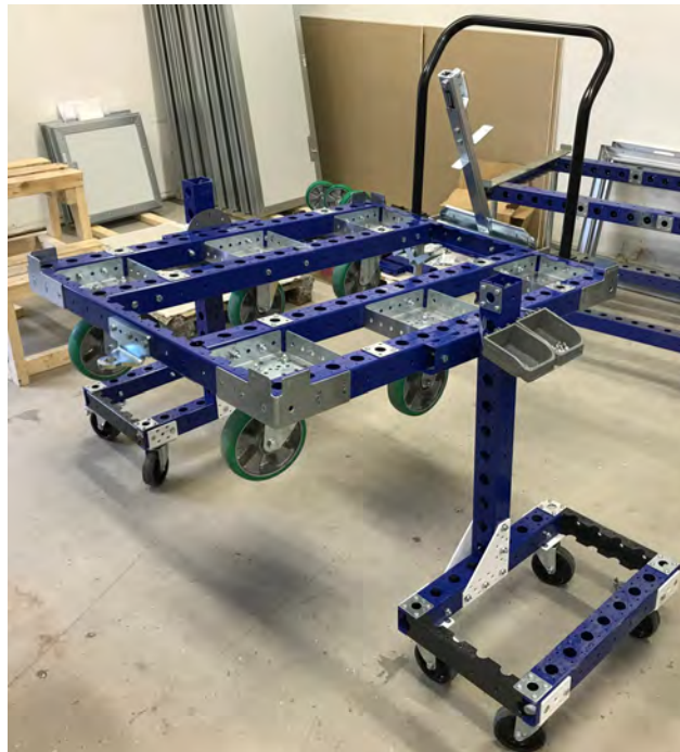
Figure 9.3: The completed cart in the rotation dollies
