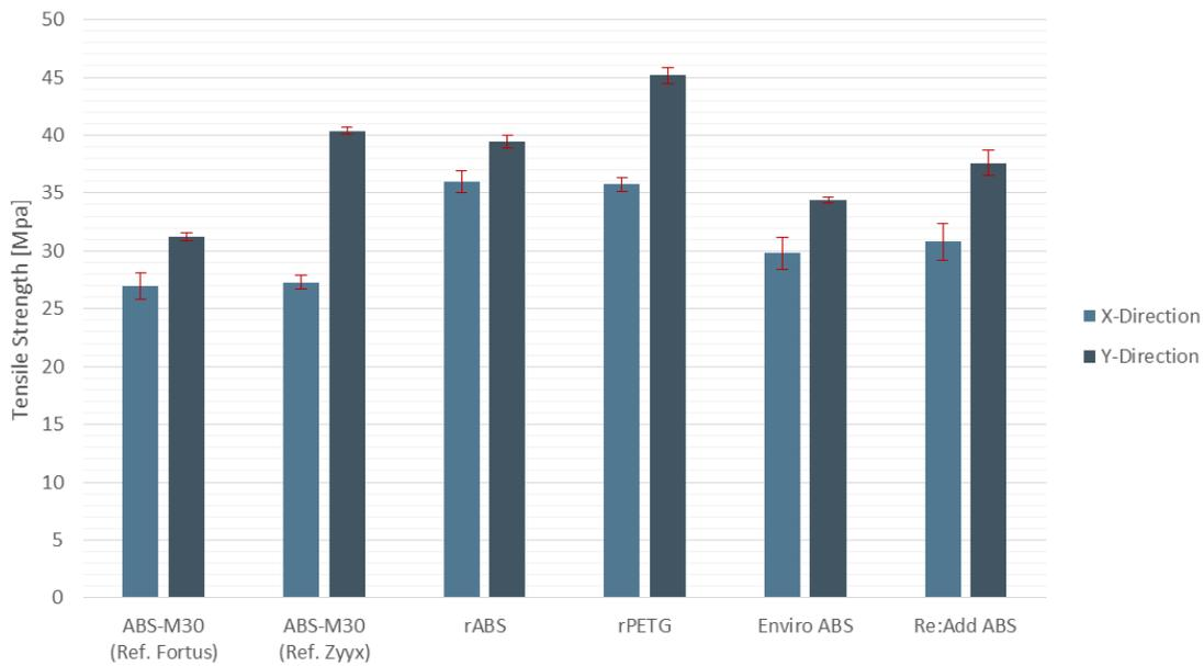
Figure 4.16: Test results of the tensile strength measurements with error bars representing 95 % confidence interval.
