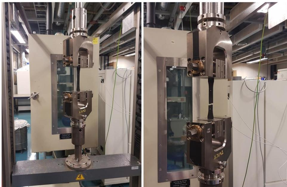
Figure 4.7: Test set-up of tensile test.
