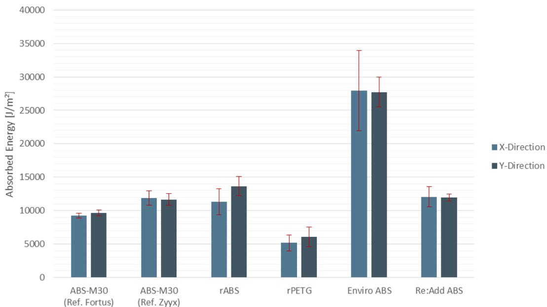
Figure 4.23: Results from impact resistance test with error bars representing 95 % confidence interval.
