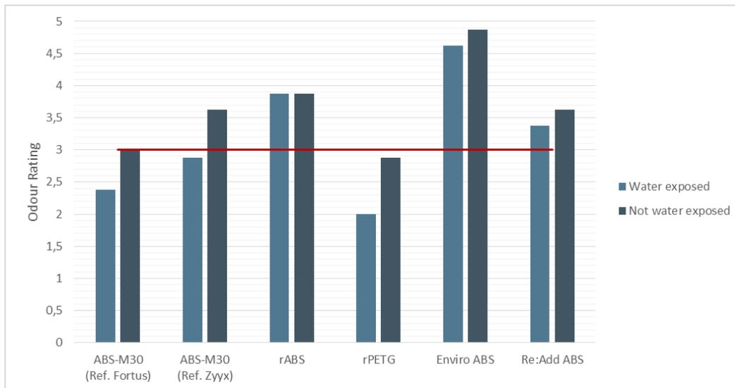
Figure 4.25: Result from odour test with maximum accepted level marked with red line.
