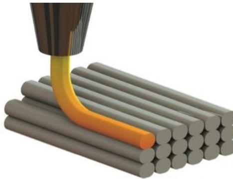
Figure 2.4: Principle illustration of the extrusion of FDM filament.
