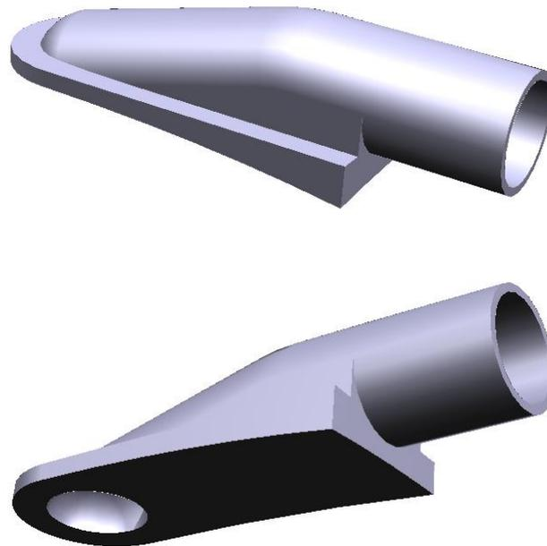
*Figure 3.1: CAD-model of the Air Duct Adapter.*
