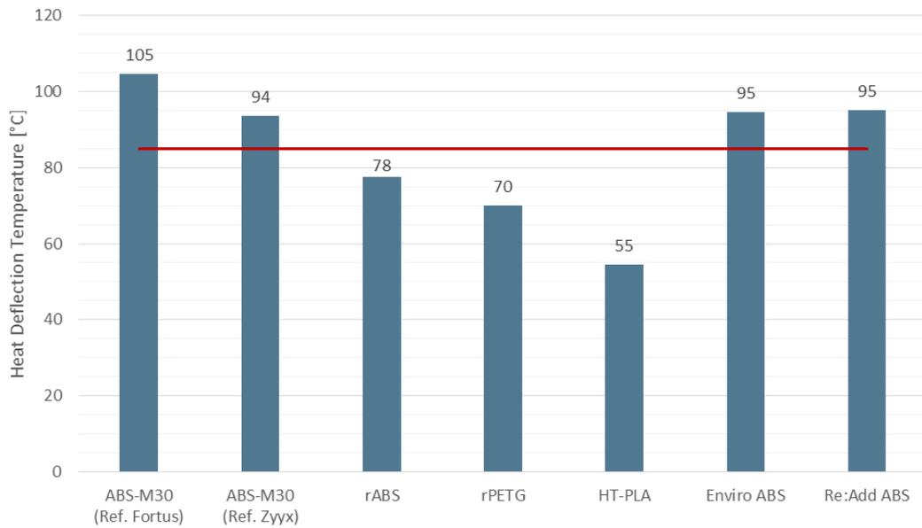
Figure 4.14: Results from HDT measurements with component temperature requirement marked in red.
