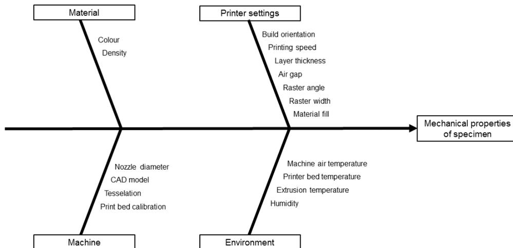
Figure 4.2: Printer parameters possibly affecting mechanical properties.
