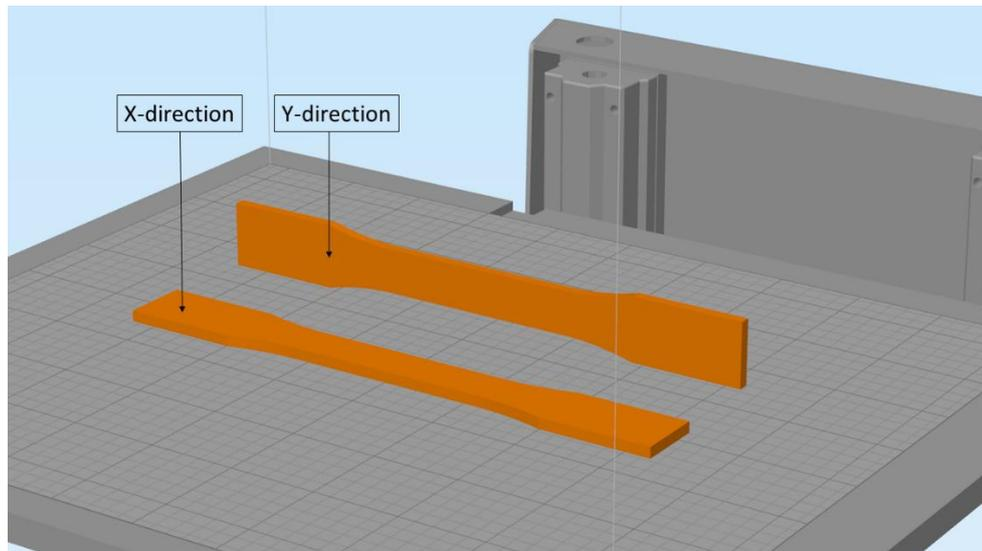
Figure 4.3: Illustration of the two printing orientations used when printing the test specimens.
