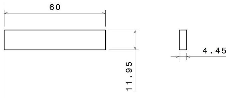
Figure 4.5: Dimensions of HDT specimen (in millimetres).
