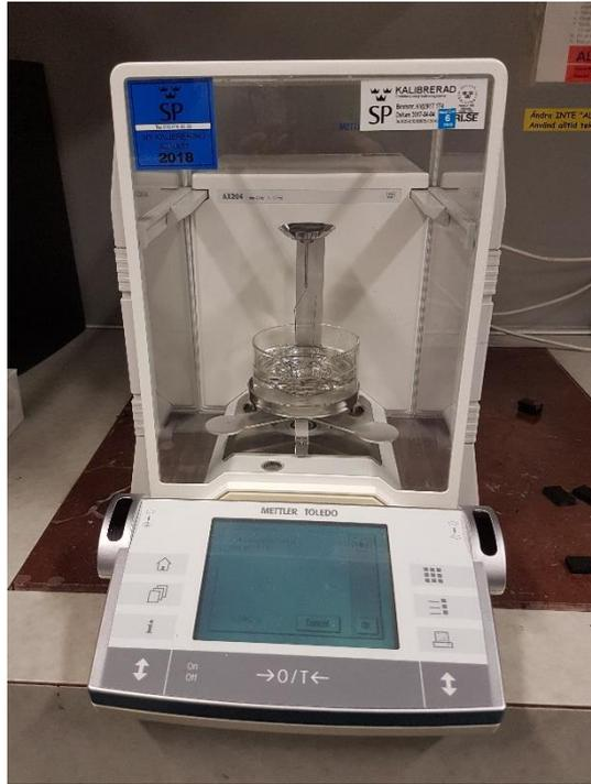
Figure 4.12: Test equipment Mettler Toledo AX204 used to measure material density.
