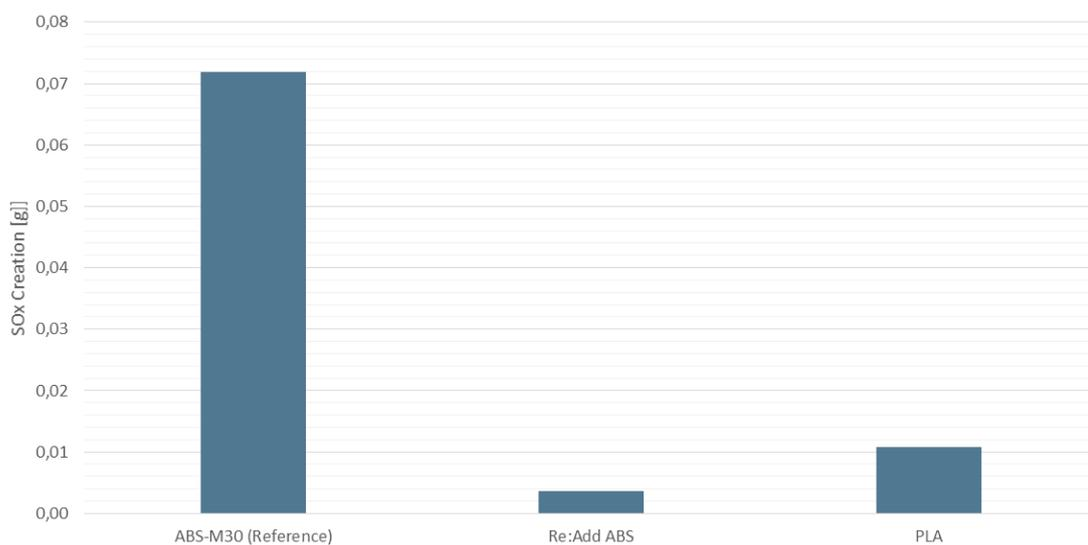
Figure 5.8: Emission of SO<sub>x</sub> from material production for each of the three materials evaluated.
