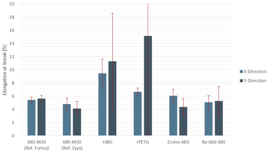
Figure 4.17: Measurements of elongation at break from tensile test with error bars representing 95 % confidence interval.
