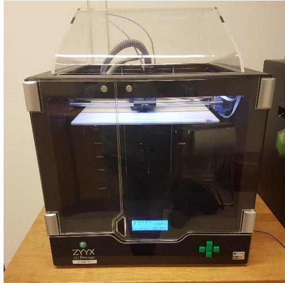
Figure 4.1: One of the three Zyx+ printers used for printing of test specimens.
