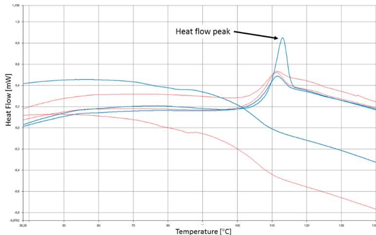
Figure 4.15: Result from DSC measurement showing the heat flow for material A (Blue curve) and material B (red curve).
