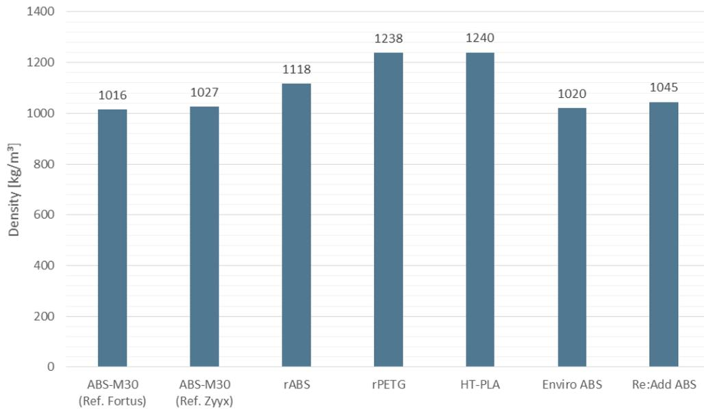
Figure 4.24: Results from density measurements.
