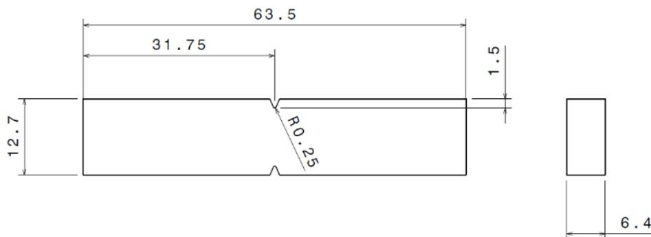
Figure 4.11: Dimensions of the pendulum impact resistance test specimen (in millimetres).
