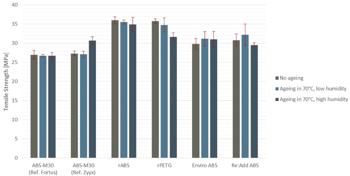
Figure 4.21: Result from tensile strength measurements comparing the materials after three different ageing procedures with error bars indicating 95% confidence interval.
