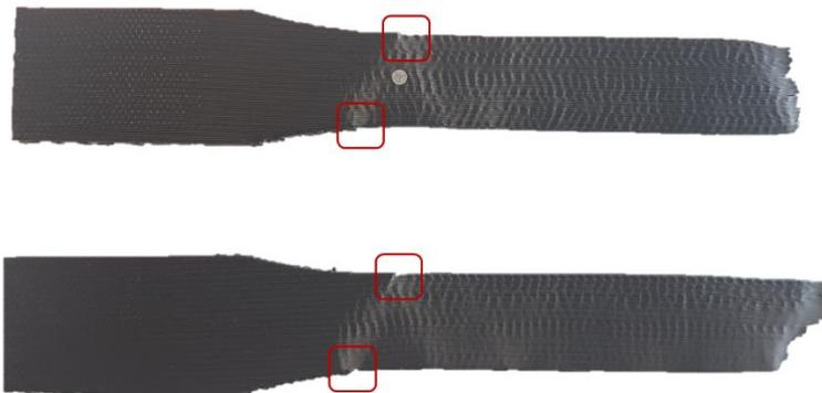
Figure 4.18: Tensile test specimens of rABS printed in Y-direction. Stress concentration areas marked in red.
