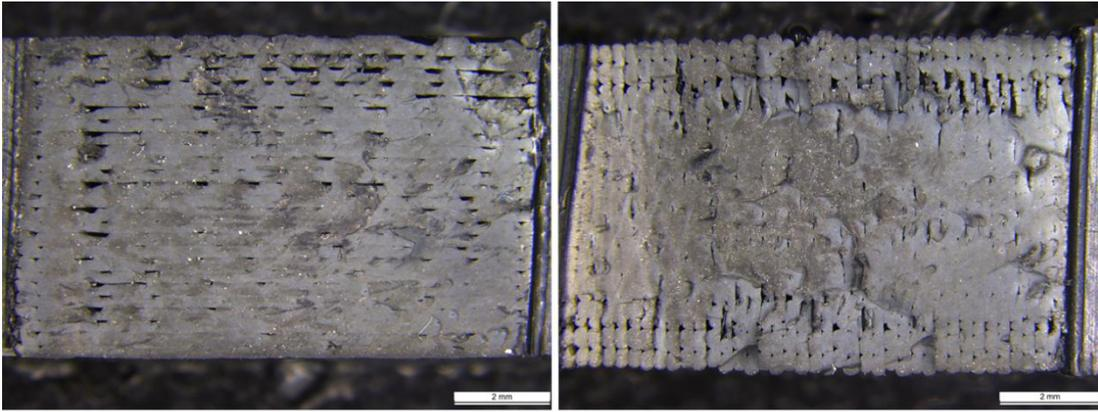
Figure 4.29: Pictures of Re:Add ABS material specimens printed in X-direction (left) and Y-direction (right).
