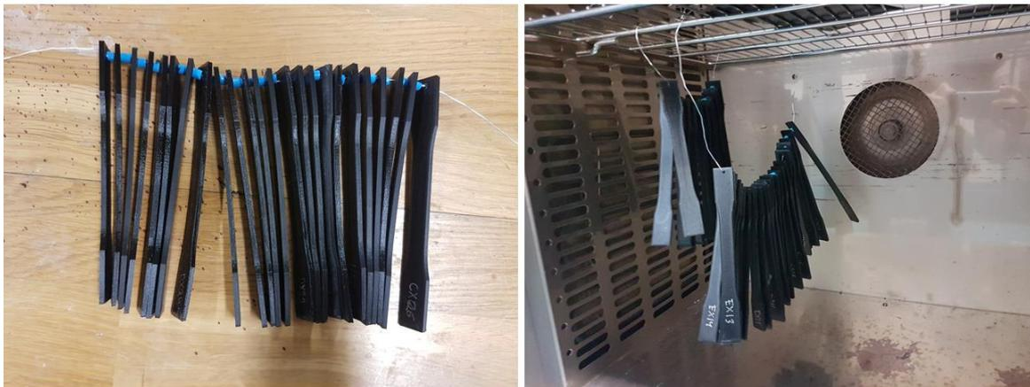
Figure 4.9: Method used for storing the specimens in ageing chambers.
