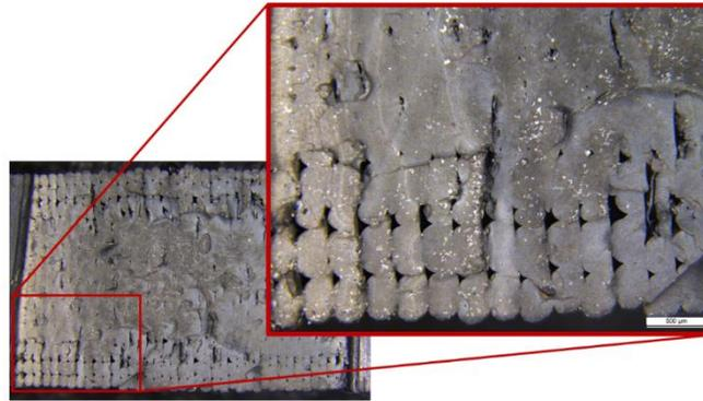
Figure 4.31: Detailed section of the Re:Add ABS material printed in Y-direction.
