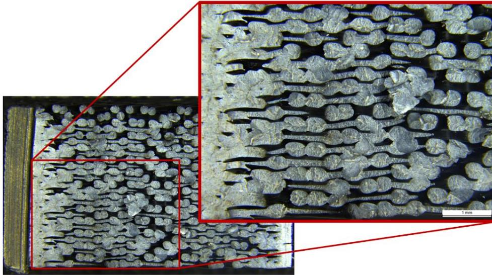
Figure 4.27: Detailed section of the Fortus reference material printed in X-direction.
