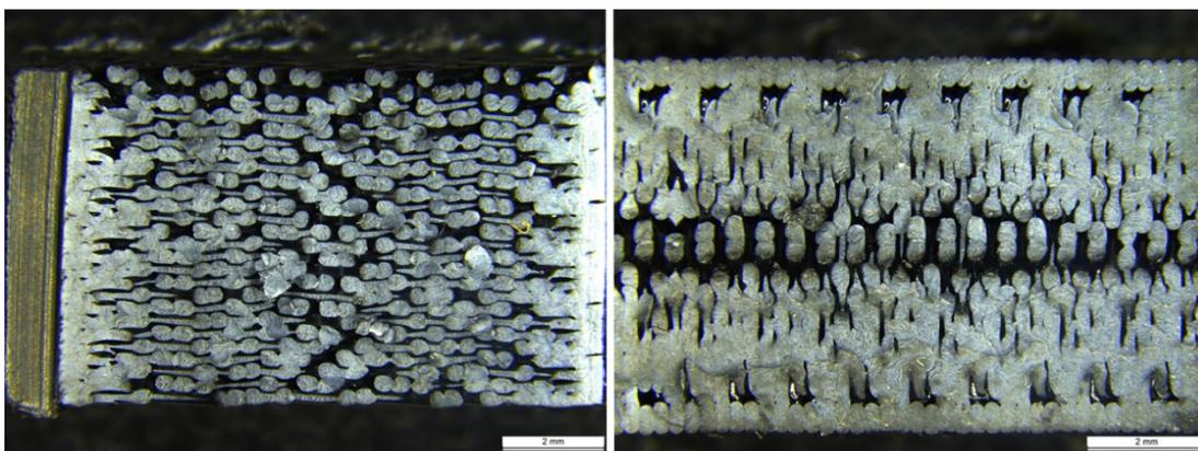
Figure 4.26: Pictures of Fortus reference specimens printed in X-direction (left) and Y-direction (right).
