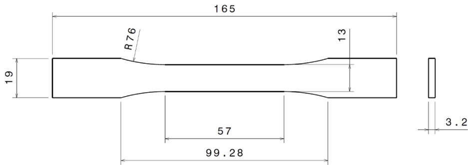
Figure 4.8: Dimensions of tensile strength specimen (in millimetres).
