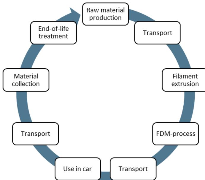
Figure 5.1: Life cycle used to calculate environmental impact of the component.
