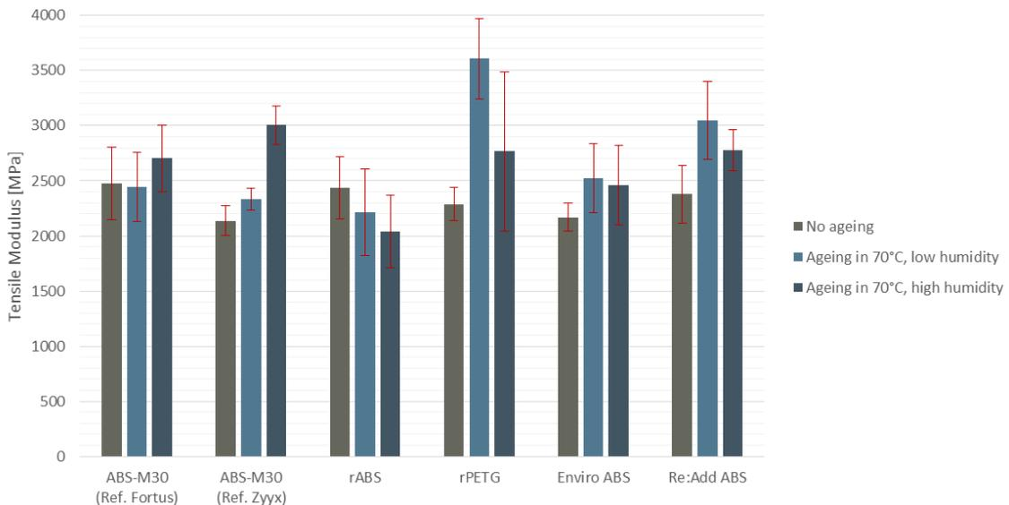
Figure 4.22: Result from tensile modulus measurements comparing the materials after three different ageing procedures with error bars indicating 95% confidence interval.
