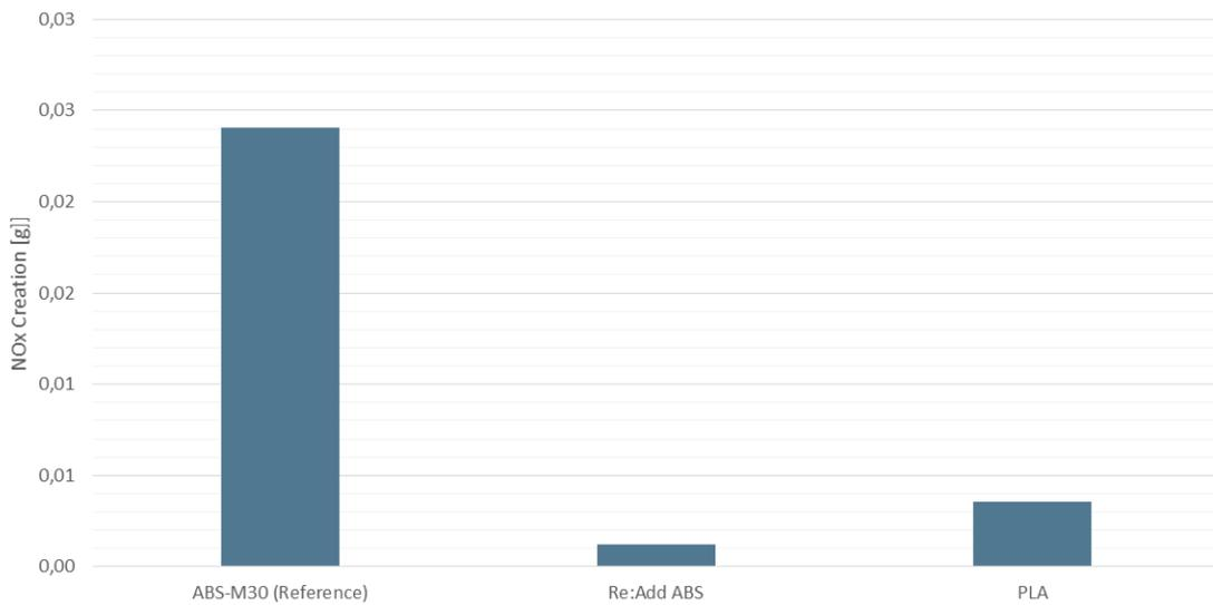
Figure 5.7: Emission of NO<sub>x</sub> from material production for each of the three materials evaluated.
