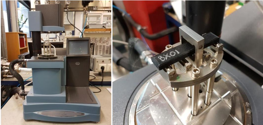
Figure 4.6: Test set-up for measuring of HDT in DMA Q800.
