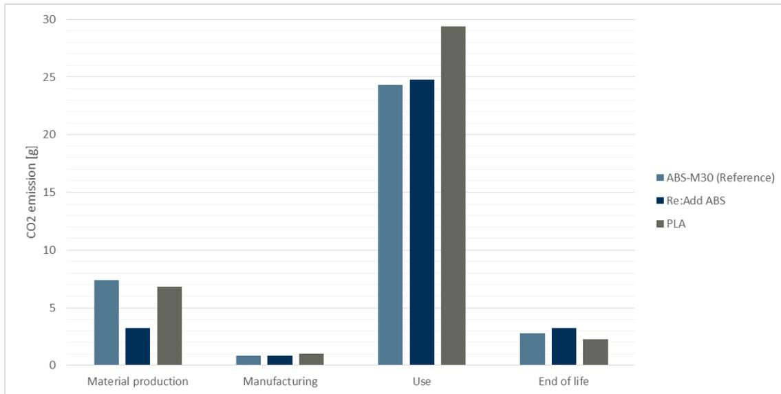
Figure 5.2: CO<sub>2</sub>-emission from each life-cycle phase for each of the three materials evaluated.
