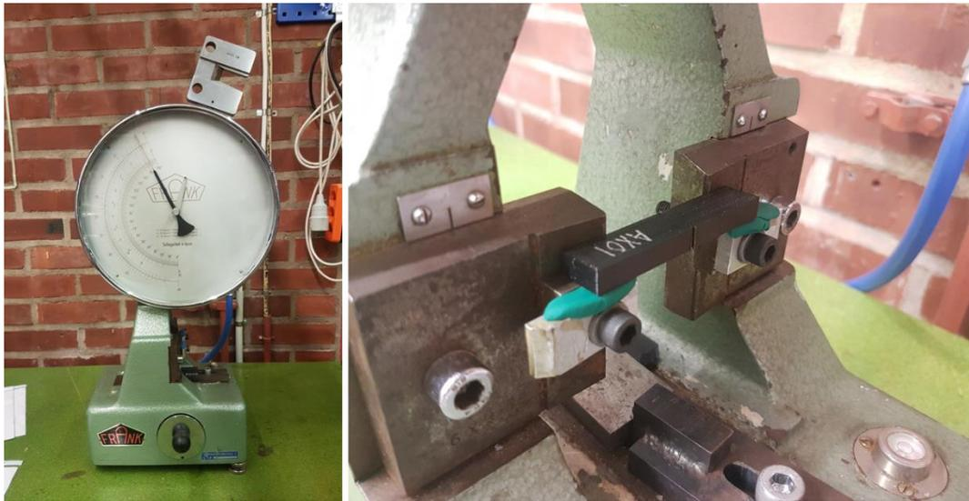
Figure 4.10: Test equipment and experiment set-up for impact resistance test, where the pendulum rotates around the scale and hits the notch of the specimen.
