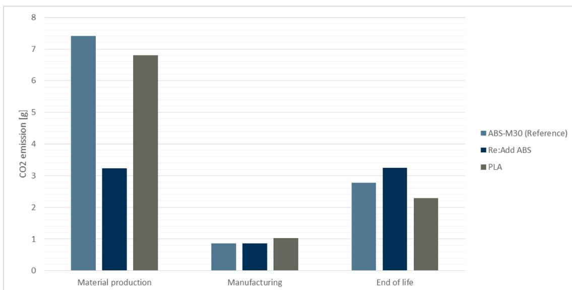
Figure 5.3: CO<sub>2</sub>-emissions for materials in each life-cycle, with the usage phase excluded.
