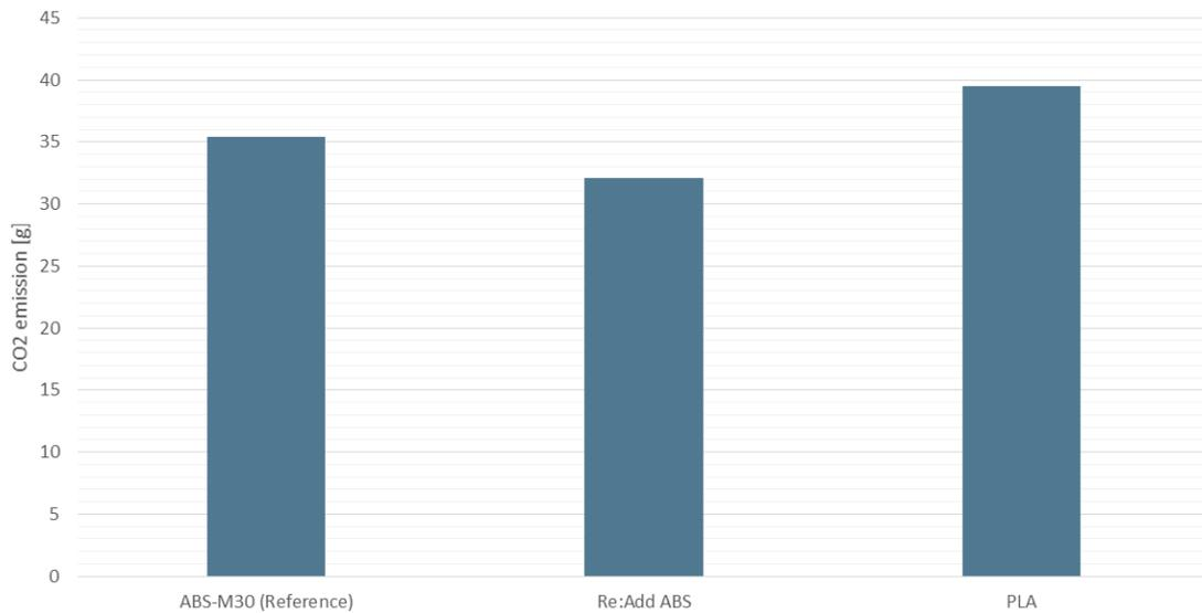
Figure 5.4: Total CO<sub>2</sub>-emission of each of the three materials including all life-cycle phases.
