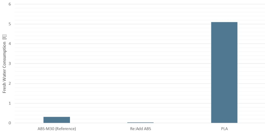
Figure 5.6: Results from calculation of fresh water consumption during material production phase.
