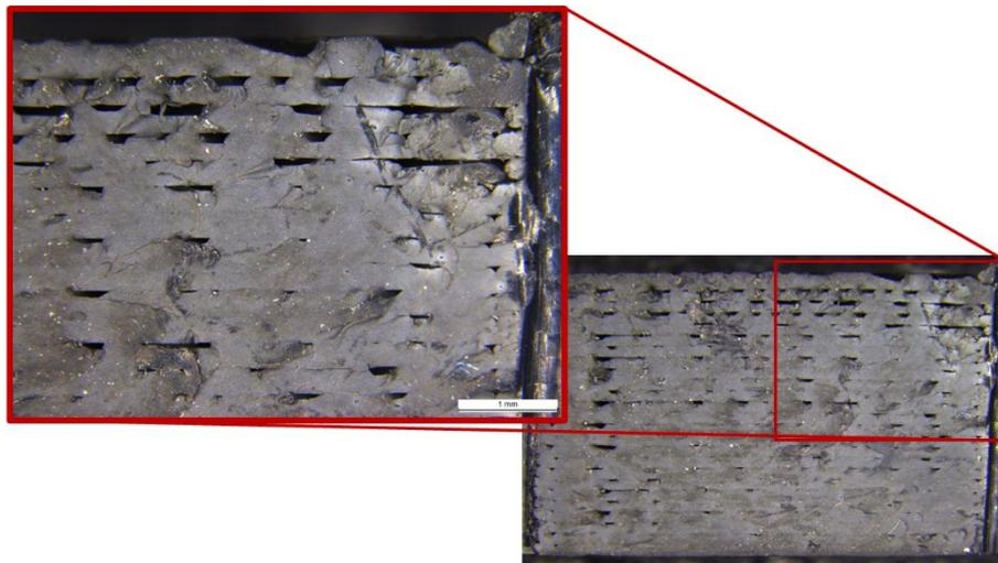
Figure 4.30: Detailed section of the Re:Add ABS material printed in X-direction.
