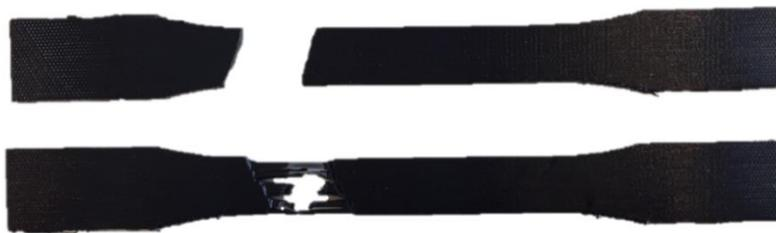
Figure 4.19: Tensile test specimens of rPETG showing a brittle fracture (upper) and a ductile fracture (lower).
