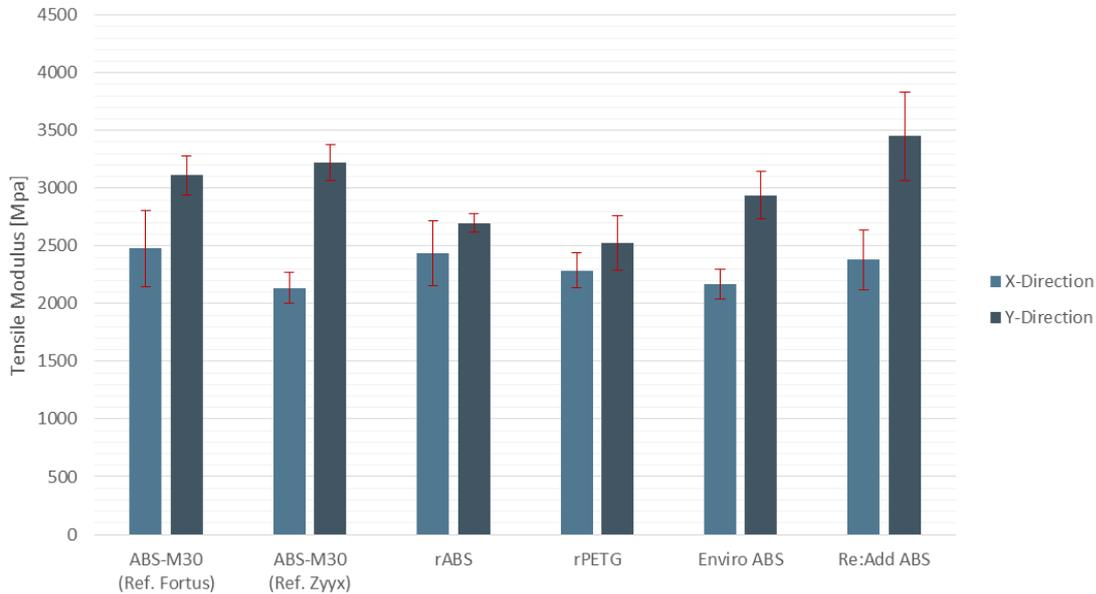
Figure 4.20: Measurements of tensile modulus with error bars representing 95 % confidence interval.
