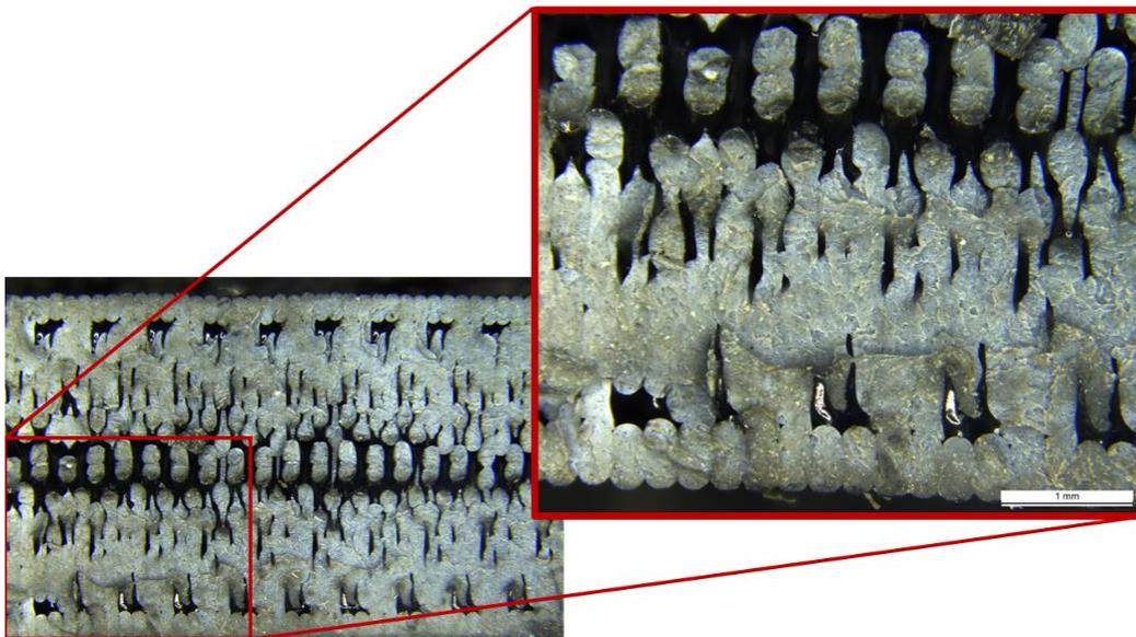
Figure 4.28: Detailed section of the Fortus reference material printed in Y-direction.
