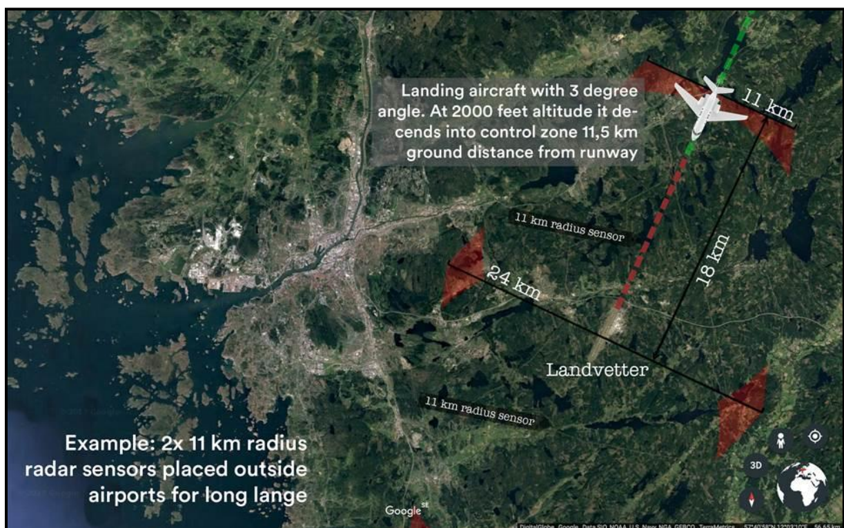
Figure 4.22 illustrates how two 11 km radius sensors more than covers the critical path of a landing aircraft in two directions.
