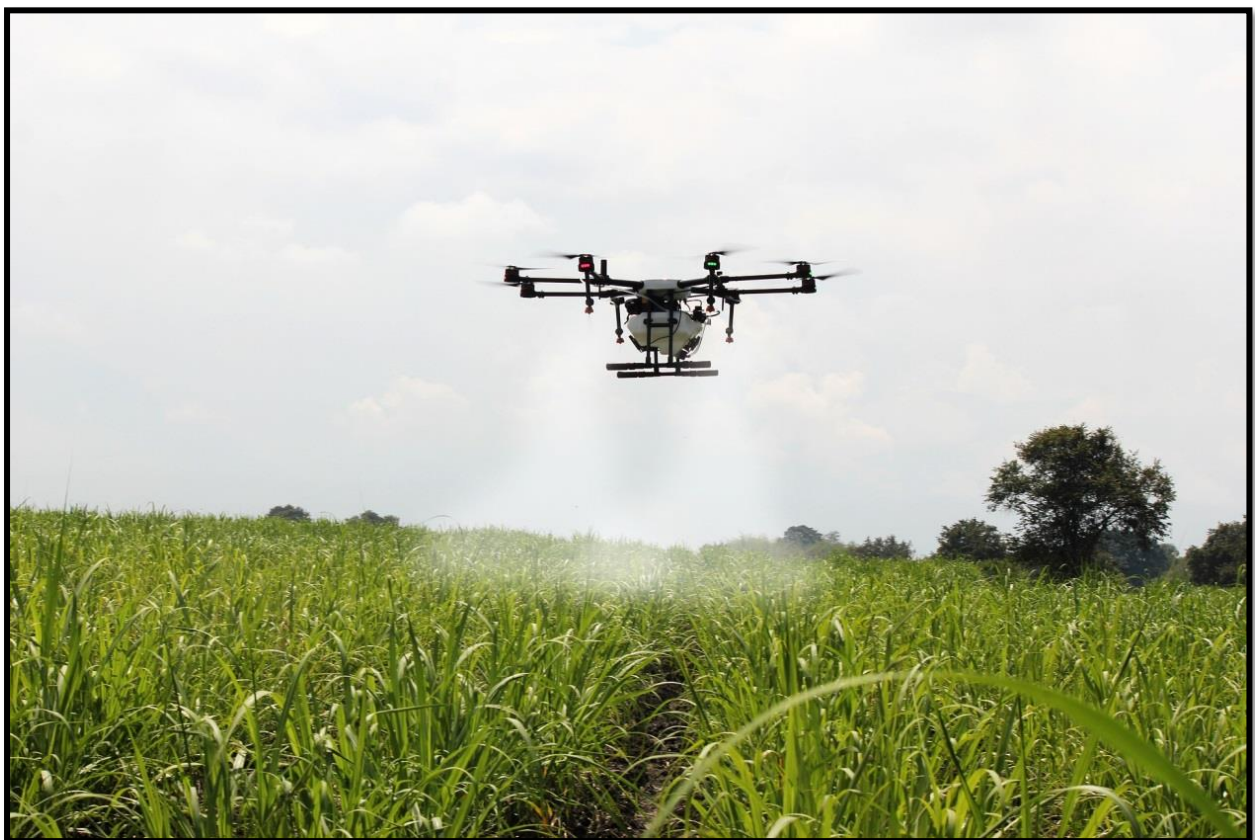
Image 4.7 shows how a DJI Agras MG-1 octocopter sprays crops with pesticide.
