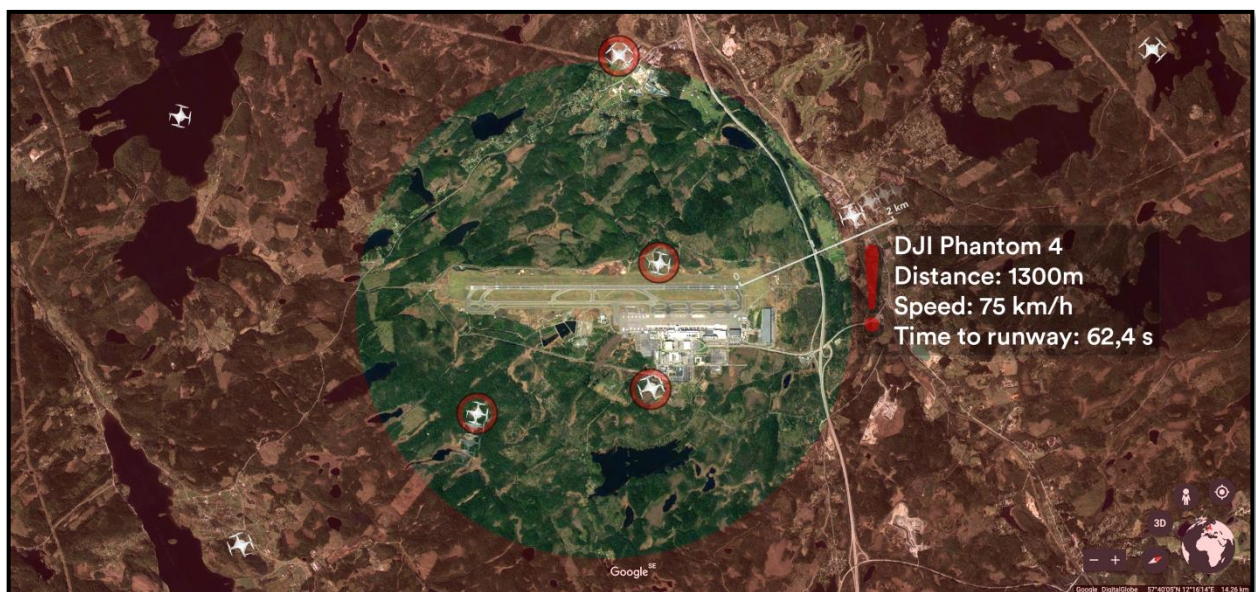
Figure 4.16 illustrates the same (as Figure 4.15) centrally placed large sensor with three kilometer radius of range.
