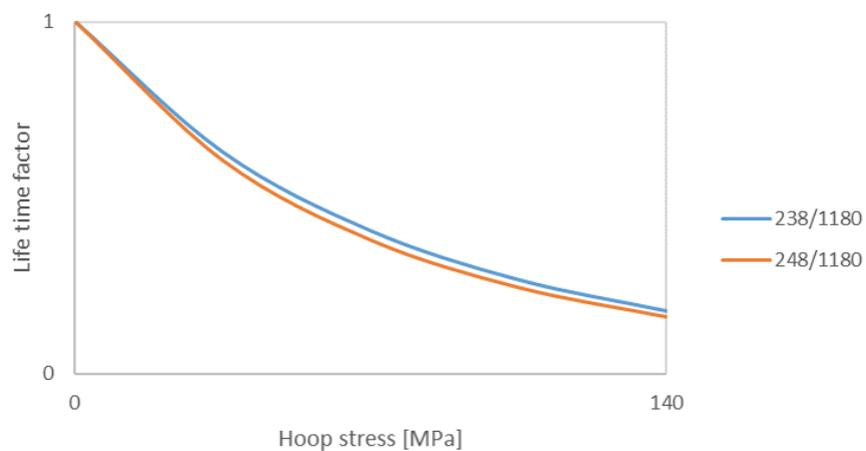
**Figure 5.15:** Shows the hoop stress effect for larger bearings with the same bore diameter of 1180 mm and a contact pressure of 1900 MPa.<sup>4</sup>
