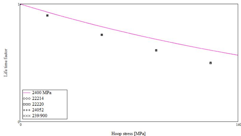
**Figure 5.20:** Shows how the meta model is performing for bearings the model was not built upon with a contact pressure of 2400 MPa.
