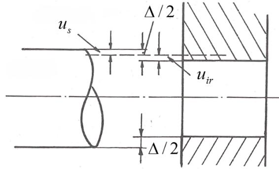
**Figure 3.5:** Shows how the interference is defined based on the displacements of the inner ring and the shaft.
