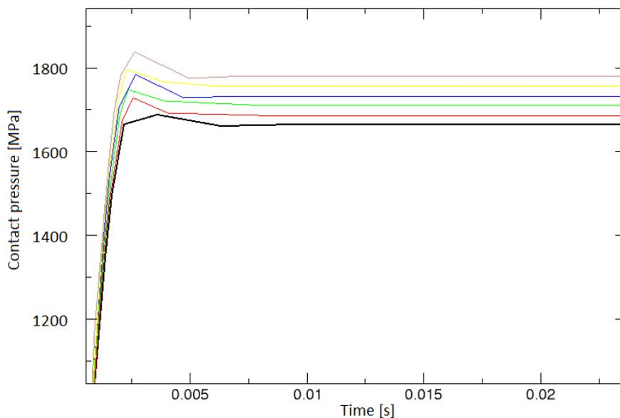
**Figure 5.16:** Shows how the contact pressure is fluctuating before the simulation stabilises and an exact value can be measured. The lines represents different loading conditions.
