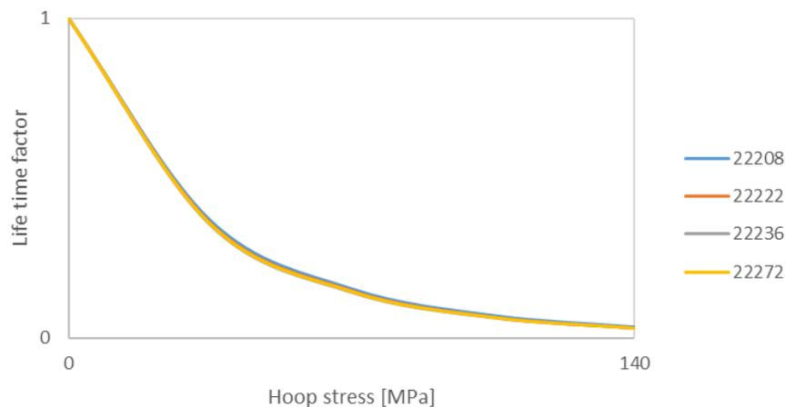
**Figure 5.10:** Shows the hoop stress effect for smaller bearings belonging to series 222 with a contact pressure of 1700 MPa.
