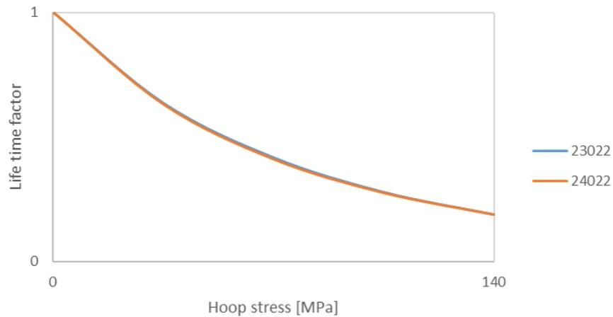
**Figure 5.14:** Shows the hoop stress effect for smaller bearings with the same bore diameter of 110 mm and a contact pressure of 1900 MPa.
