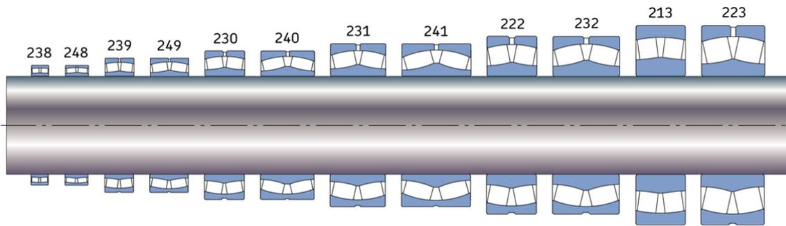
**Figure 3.1:** The figure shows how the series are varying for the same bore diameter.
