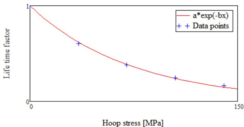
**Figure 5.6:** Shows the curve fit of the hoop stress effect on the life time factor for bearing 24072.
