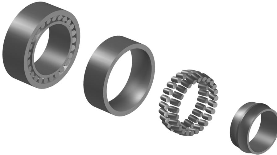
**Figure 3.3:** Shows the interface of BEAST when a complete bearing has been assembled together with an exploded view of the same.
