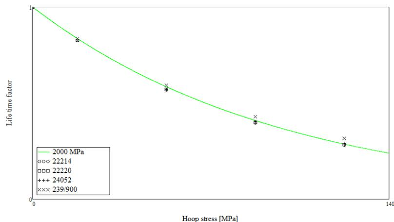
**Figure 5.19:** Shows how the meta model is performing for bearings the model was not built upon with a contact pressure of 2000 MPa.
