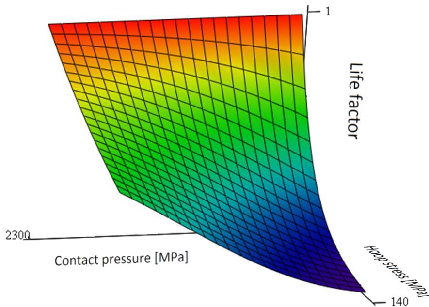
**Figure 5.8:** Shows the surface which describes the life time factor as a function of the hoop stress and the contact pressure for bearing 24072.
