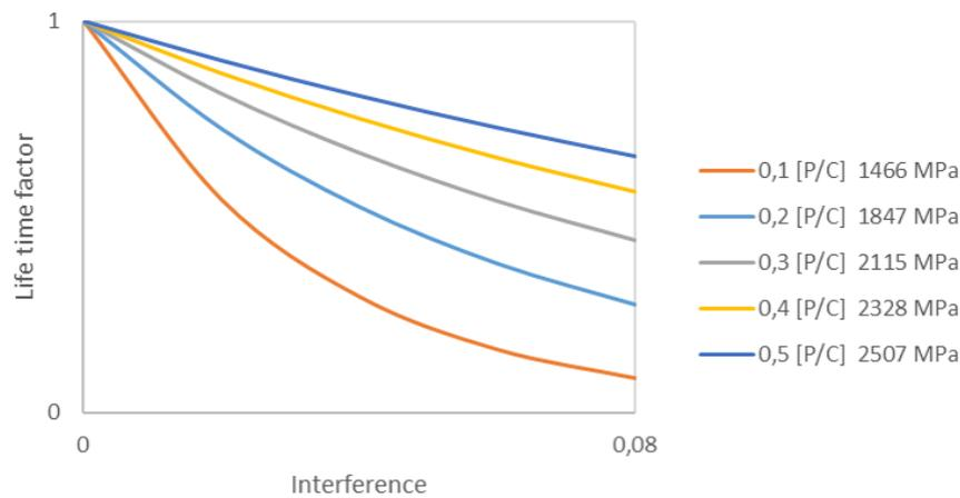
**Figure 5.23:** Shows the evaluation of bearing 22372 at the set engineering levels of load and interference.
