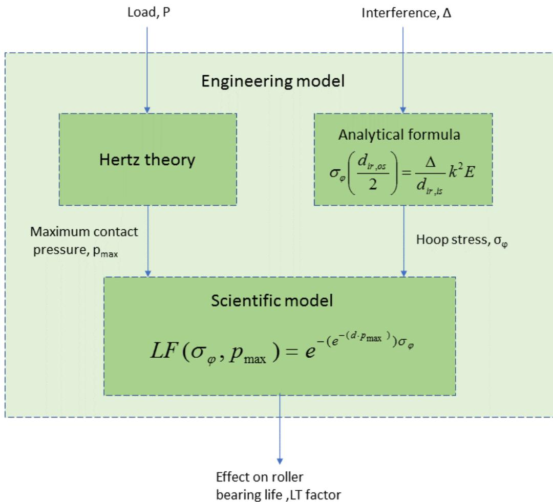
**Figure 5.28:** Shows the principles of the final meta model for the engineering level.
