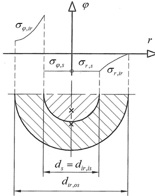
**Figure 3.4:** Shows the stress distribution through the ring and the shaft [2].
