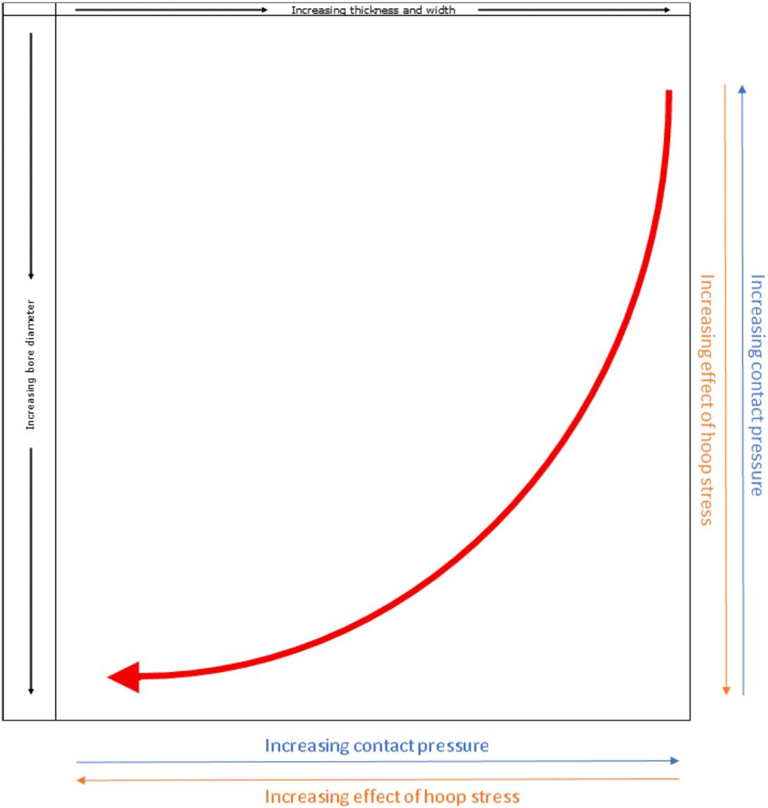
**Figure A.17:** Shows the behaviour of the contact pressure and the hoop stress over the assortment. The red arrow shows the direction of increasing effect of hoop stress. The assortment matrix is modified due to confidentiality.
