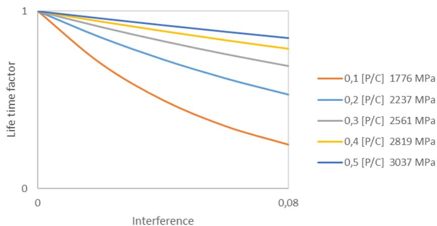
**Figure 5.22:** Shows the evaluation of bearing 22308 at the set engineering levels of load and interference.
