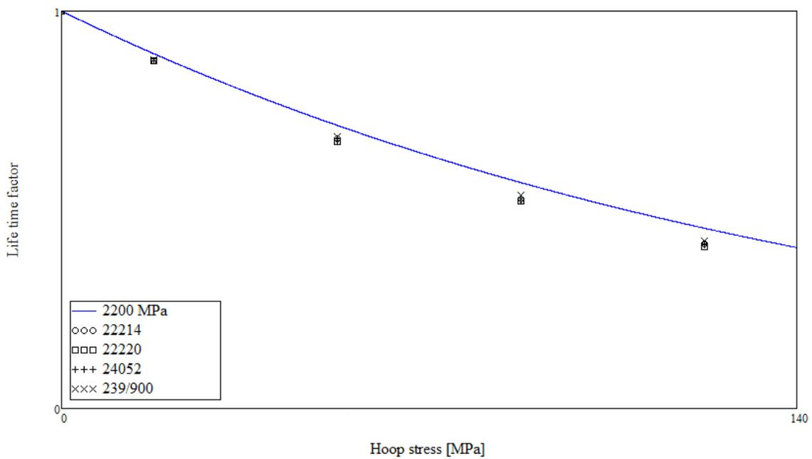
**Figure A.15:** Shows how the meta model is performing for bearings the model was not built upon with a contact pressure of 2200 MPa.
