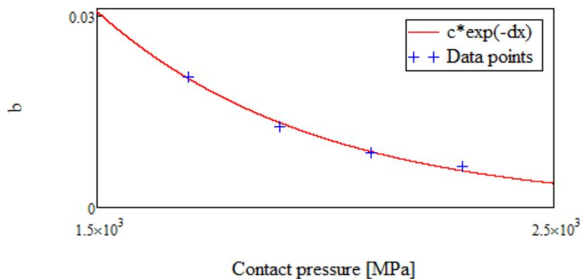
**Figure 5.7:** Shows the curve fit of the contact pressure effect in regard to the  $b$  values.
