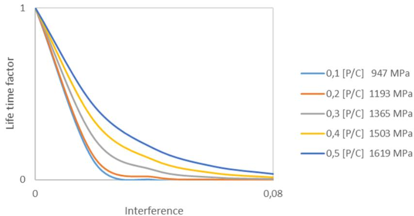
**Figure 5.25:** Shows the evaluation of bearing 238/1180 at the set engineering levels of load and interference.
