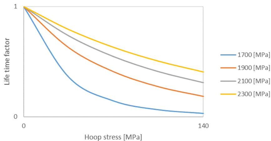
**Figure 5.2:** Shows the life time factor plotted against the hoop stress, with fixed levels of contact pressure for bearing 24072.
