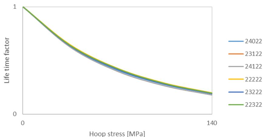
**Figure 5.12:** Shows the hoop stress effect for bearings with a bore diameter of 110 mm and a contact pressure of 1900 MPa.
