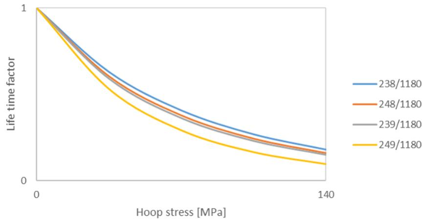
**Figure 5.13:** Shows the hoop stress effect for bearings with a bore diameter of 1180 mm and a contact pressure of 1900 MPa.<sup>3</sup>
