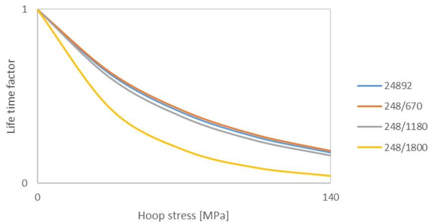
**Figure 5.11:** Shows the hoop stress effect for larger bearings belonging to series 248 with a contact pressure of 1900 MPa.<sup>2</sup>
