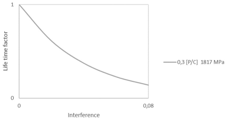
**Figure 5.26:** Shows the evaluation of bearing 241/670 at the set engineering levels of load and interference.
