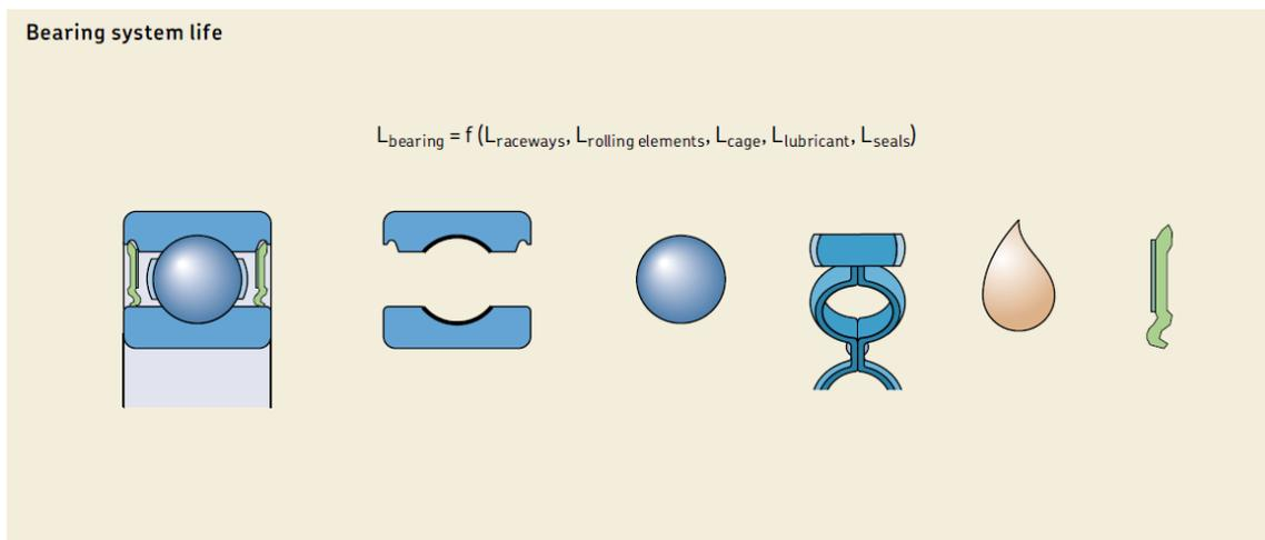
**Figure 3.2:** Shows the factors affecting the life time of a bearing as a system [3].
