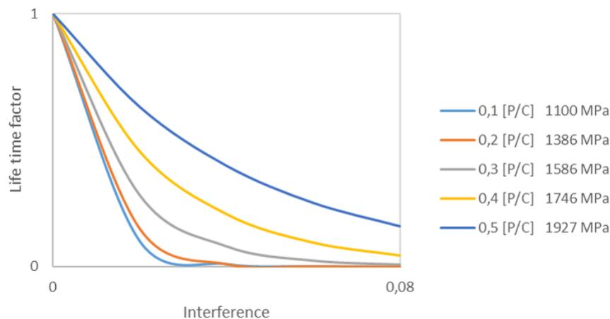
**Figure 5.24:** Shows the evaluation of bearing 23972 at the set engineering levels of load and interference.
