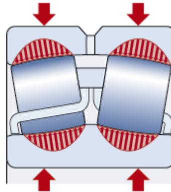
**Figure 1.2:** Shows the load distribution on the rollers during contact with the inner and outer ring [3].
