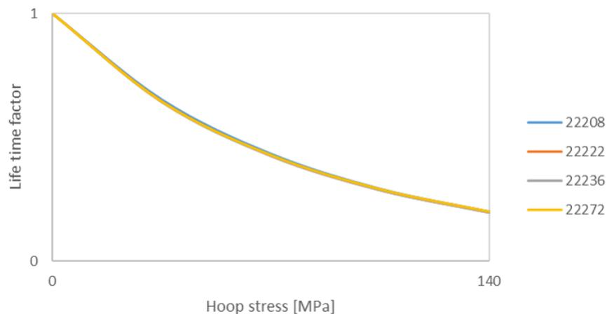
**Figure 5.9:** Shows the hoop stress effect for smaller bearings belonging to series 222 with a contact pressure of 1900 MPa.
