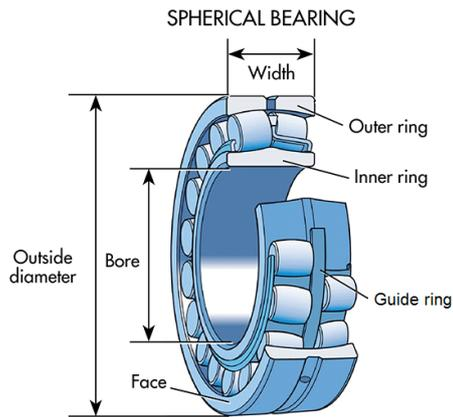
**Figure 1.1:** Shows the compound of a spherical roller bearing with included part denomination [1].
