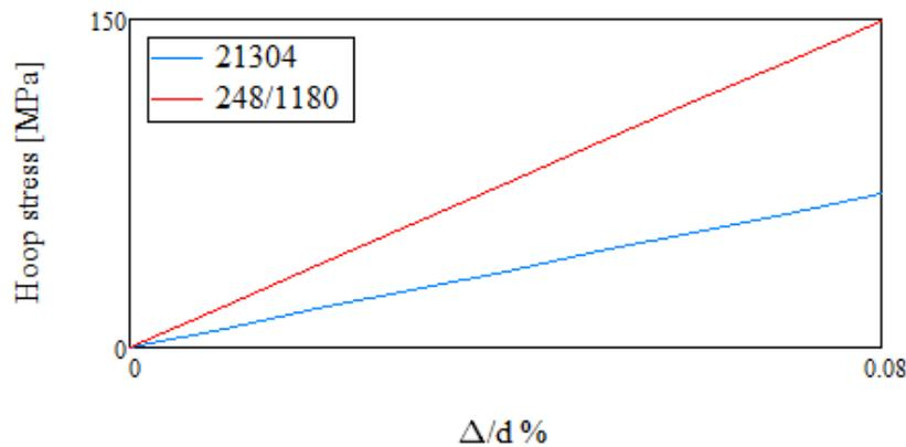
**Figure 5.21:** Shows the hoop stress levels increase with increasing  $\Delta/d$  for the bearings 21304 and 248/1180.
