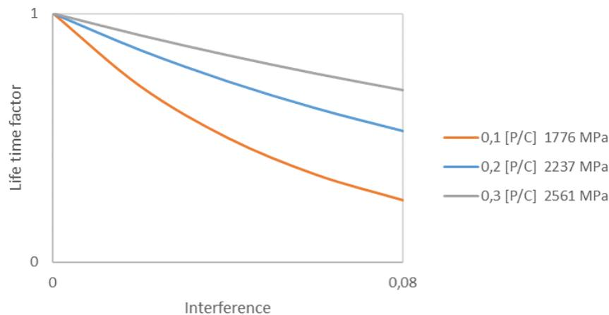
**Figure 5.27:** Shows the evaluation of bearing 22308 at the set engineering levels of load and interference.
