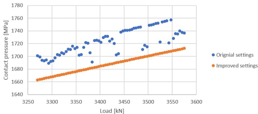
**Figure 5.17:** Shows how the contact pressure is differing between the two cases of settings for bearing 232/670.
