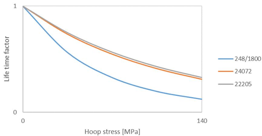
**Figure 5.3:** Shows the life time factor plotted against the hoop stress, with 2100 MPa of contact pressure for all of the three bearings.<sup>1</sup>
