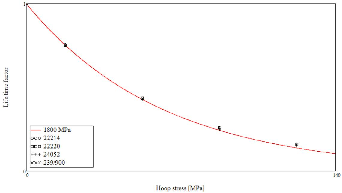
**Figure A.14:** Shows how the meta model is performing for bearings the model was not built upon with a contact pressure of 1800 MPa.
