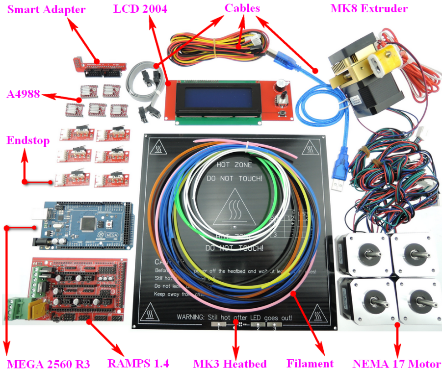
Figure 5.1: Cartesian 3D printer Hardware Components
