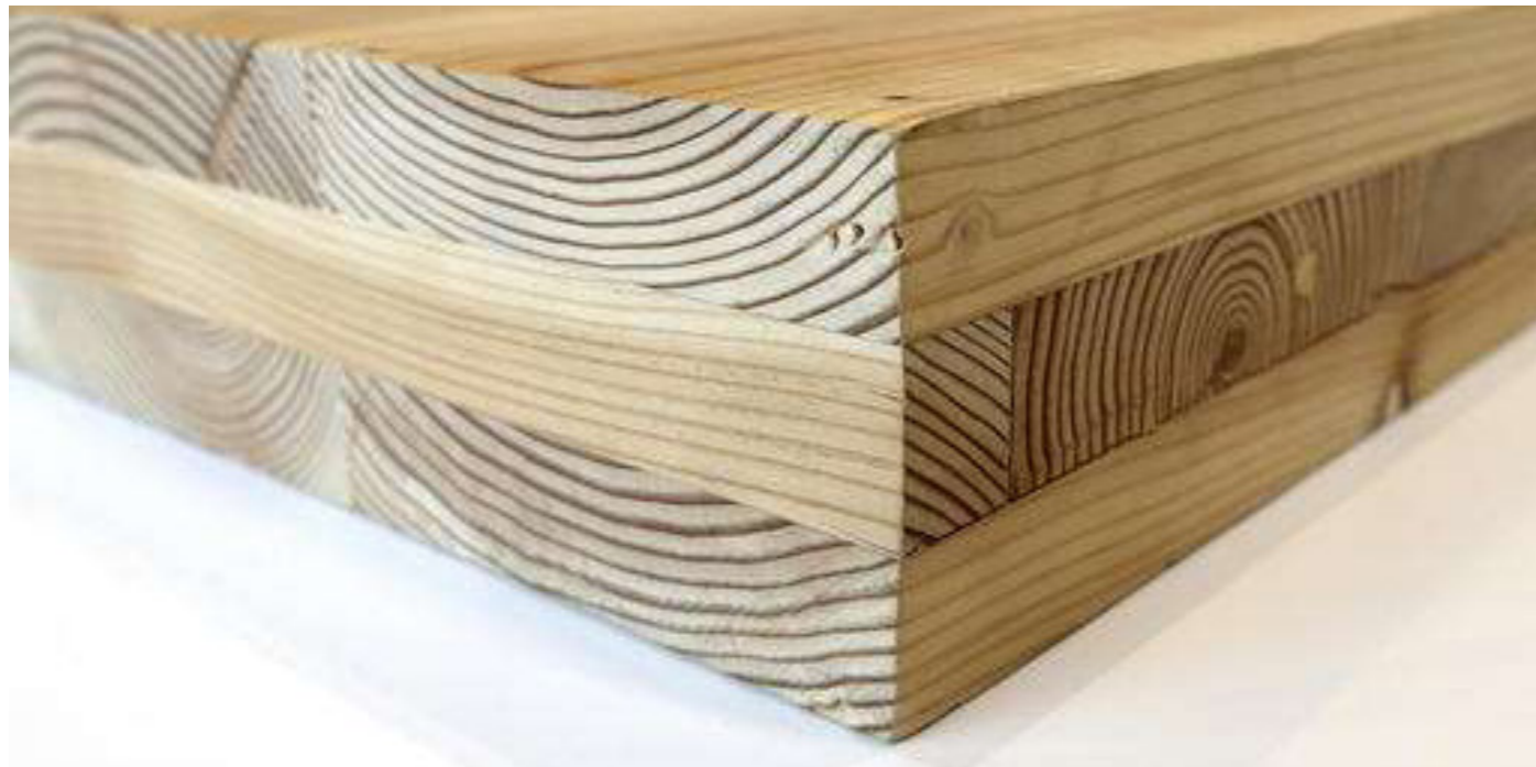
Figure 9. CLT is made up of 2-by-4 beams laid out in perpendicular layers that are then glued together to make giant panels. (Don Ryan).
