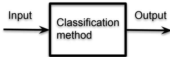
Figure 1.2: High level sketch of the classification pipeline. Radar data, images and the two combined will serve as input. The classification method is either a neural network or a support vector machine and the output is the assigned class of the corresponding input.
