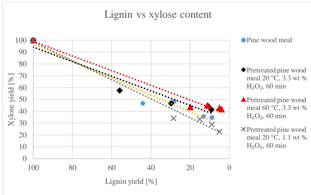
Figure 15: Results of xylose yield as a function of the delignification for the pine wood samples during soda pulping.
