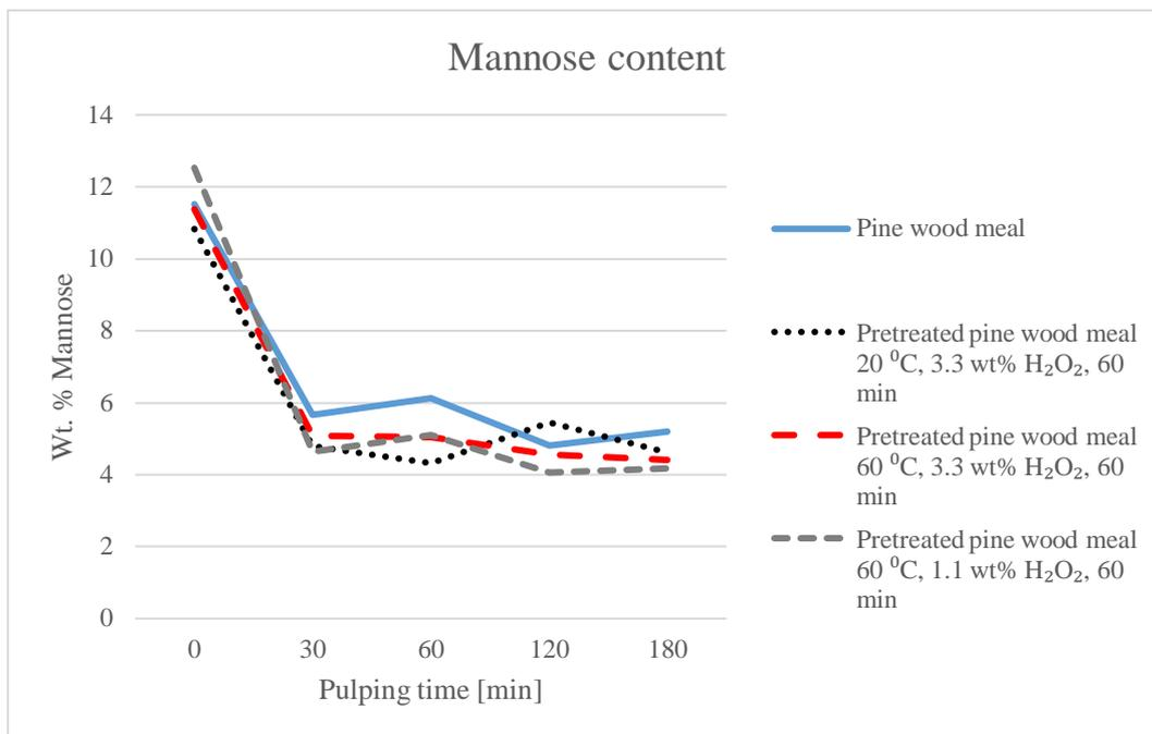
Figure 14: Results of mannose content in weight percentage after alkaline hydrogen peroxide pretreatment followed by soda pulping of pine wood meal. The zero-point on the x-axis shows the values prior to the warm-up period, the other times are set after the warm-up period.
