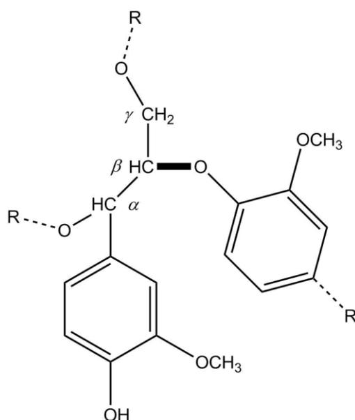
Figure 6: Illustration of the  $\beta$ -O-4 bond (bold) between two lignin monomers.
