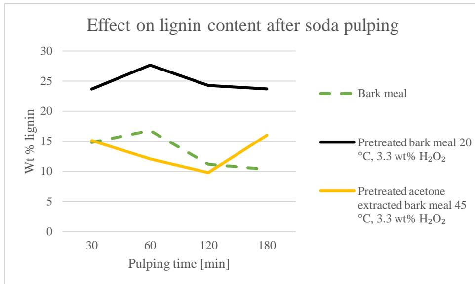
Figure 17: Results of Klason lignin content in weight percentage after alkaline hydrogen peroxide pretreatment followed by soda pulping of bark meal.
