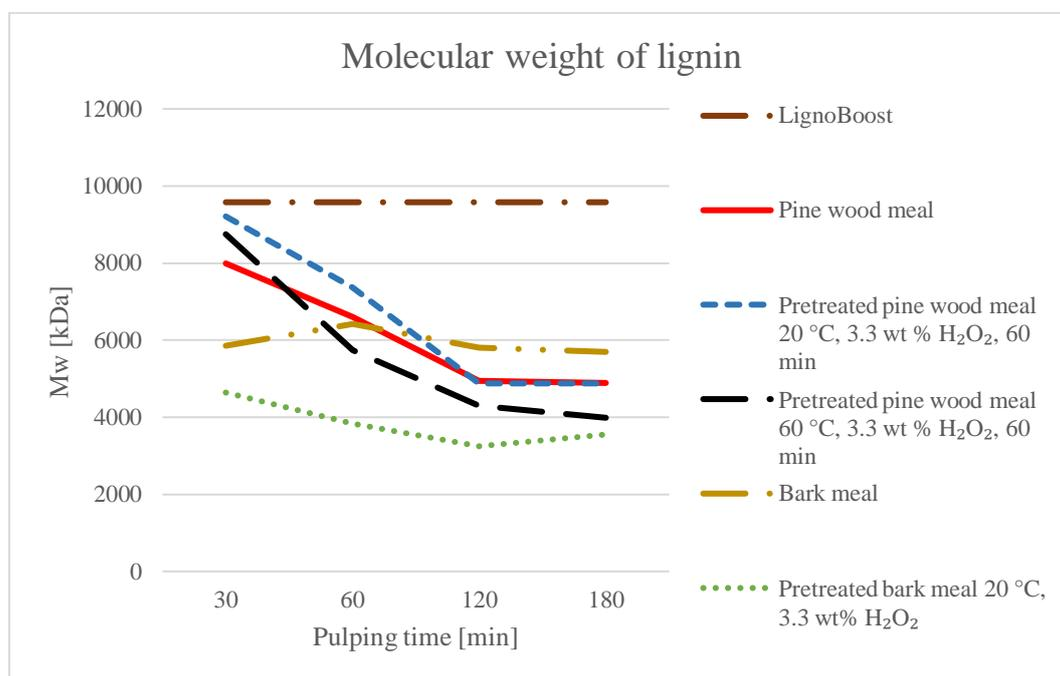
Figure 18: Molecular weight of lignin for the different samples of pine wood meal and bark meal using LignoBoost softwood Kraft lignin from Bäckhammar as reference.
