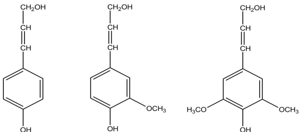
Figure 5: Molecular structure of the three lignin monomers units. From left to right: *p*-coumaryl alcohol, sinapyl alcohol and coniferyl alcohol.
