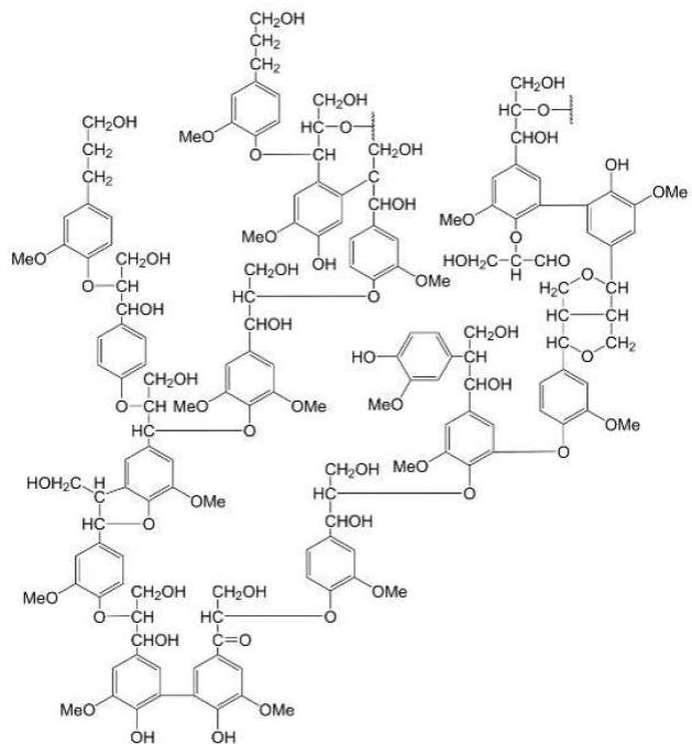
*Figure 4: Proposed structure of softwood lignin. Adapted from Adler (1977).*
