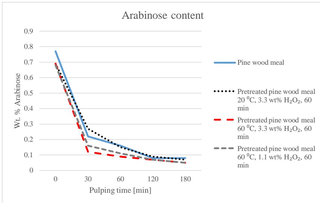
Figure 12: Results of arabinose content in weight percentage after alkaline hydrogen peroxide pretreatment followed by soda pulping of pine wood meal. The zero-point on the x-axis shows the values prior to the warm-up period, the other times are set after the warm-up period.
