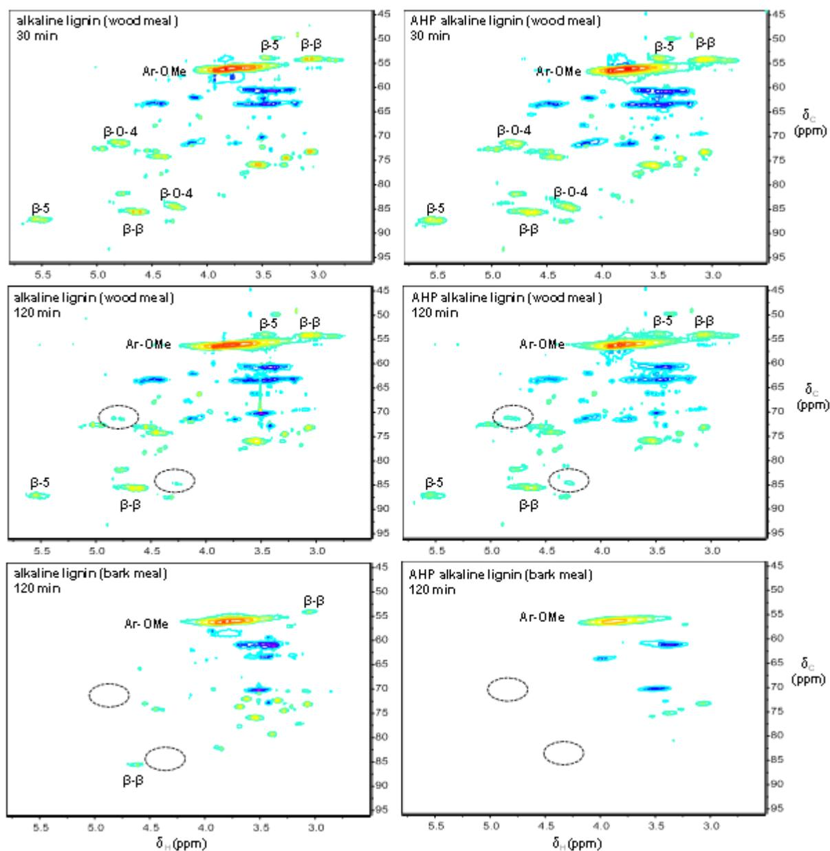
Figure 25: The Inter-unit aliphatic lignin region/oxygenated aliphatic region  $\delta_C/\delta_H$  44-96/2.5-5.2 ppm of 2D NMR spectra (800 MHz, DMSO-d<sub>6</sub>) of untreated and AHP pretreated alkaline lignin from pine wood and softwood bark.
