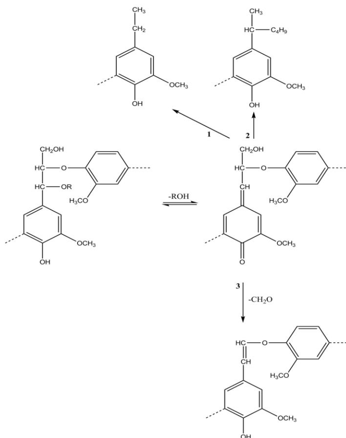
Figure 8: Illustration of the different reaction of phenolic  $\beta$ -O-4 structures in lignin. Reduction reaction (1), condensation reaction (2) and elimination reaction into an enol ether from quinone methide (3).
