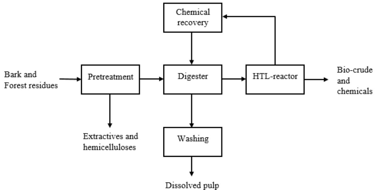
*Figure 10: Flowsheet for the proposed forest residue biorefinery.*
