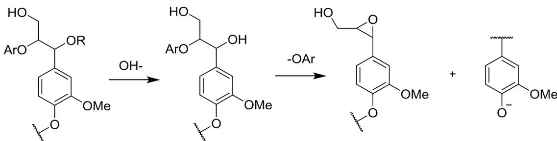
Figure 7: Illustration of cleavage of non-phenolic  $\beta$ -O-4 structures in lignin.
