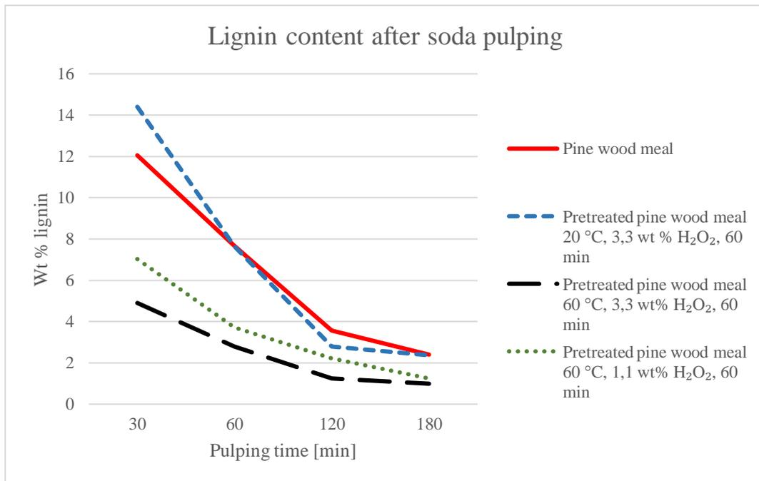
Figure 16: Results of Klason lignin content in weight percentage after alkaline hydrogen peroxide pretreatment followed by soda pulping of pine wood meal.
