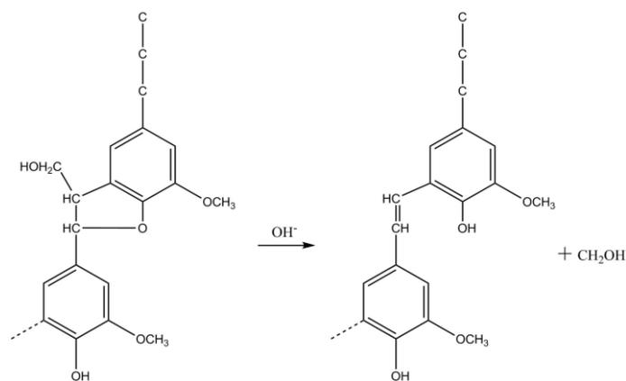
Figure 9: Illustration of  $\beta$ -5 lignin bond reaction under alkaline conditions.
