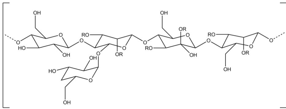
Figure 2: Molecular structure of a softwood glucomannan unit.
