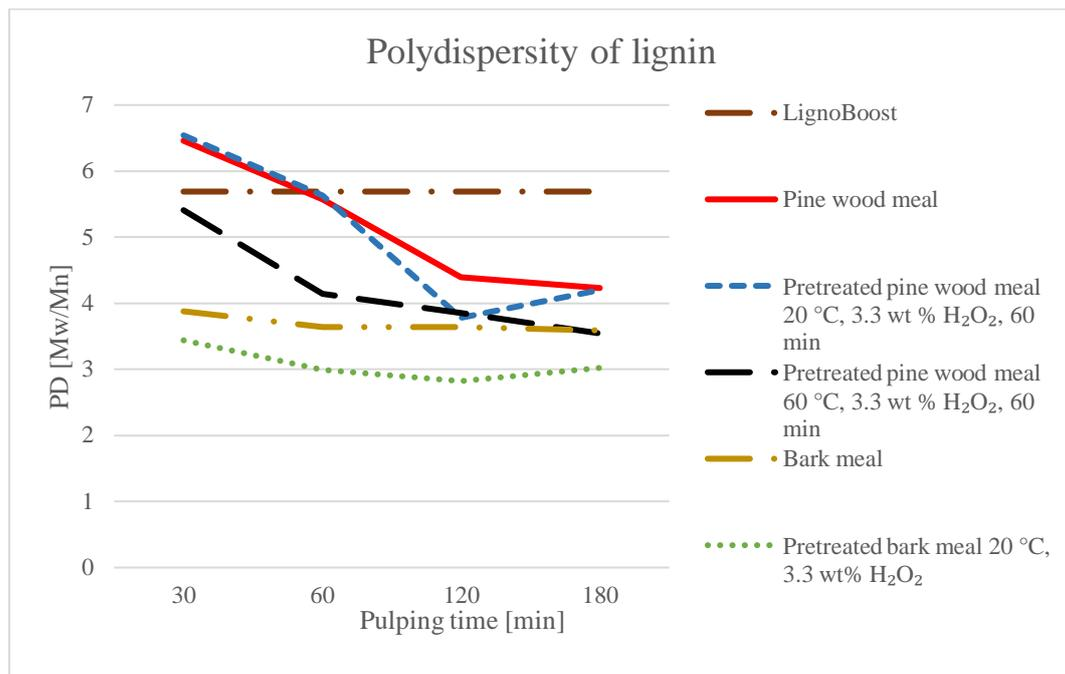
Figure 19: Result for polydispersity of lignin for the different samples of pine wood meal and bark meal using LignoBoost softwood Kraft lignin from Bäckhammar as reference.
