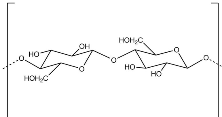
*Figure 1: Molecular structure of a cellulose unit.*
