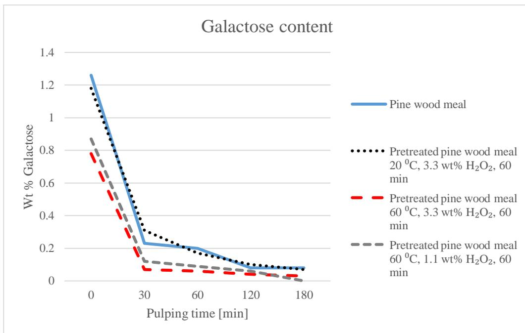
Figure 13: Results of galactose content in weight percentage after alkaline hydrogen peroxide pretreatment followed by soda pulping of pine wood meal. The zero-point on the x-axis shows the values prior to the warm-up period, the other times are set after the warm-up period.
