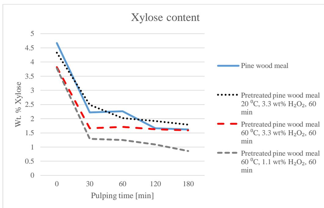
Figure 11: Results of xylose content in weight percentage after alkaline hydrogen peroxide pretreatment followed by soda pulping of pine wood meal. The zero-point on the x-axis shows the values prior to the warm-up period, the other times are set after the warm-up period.
