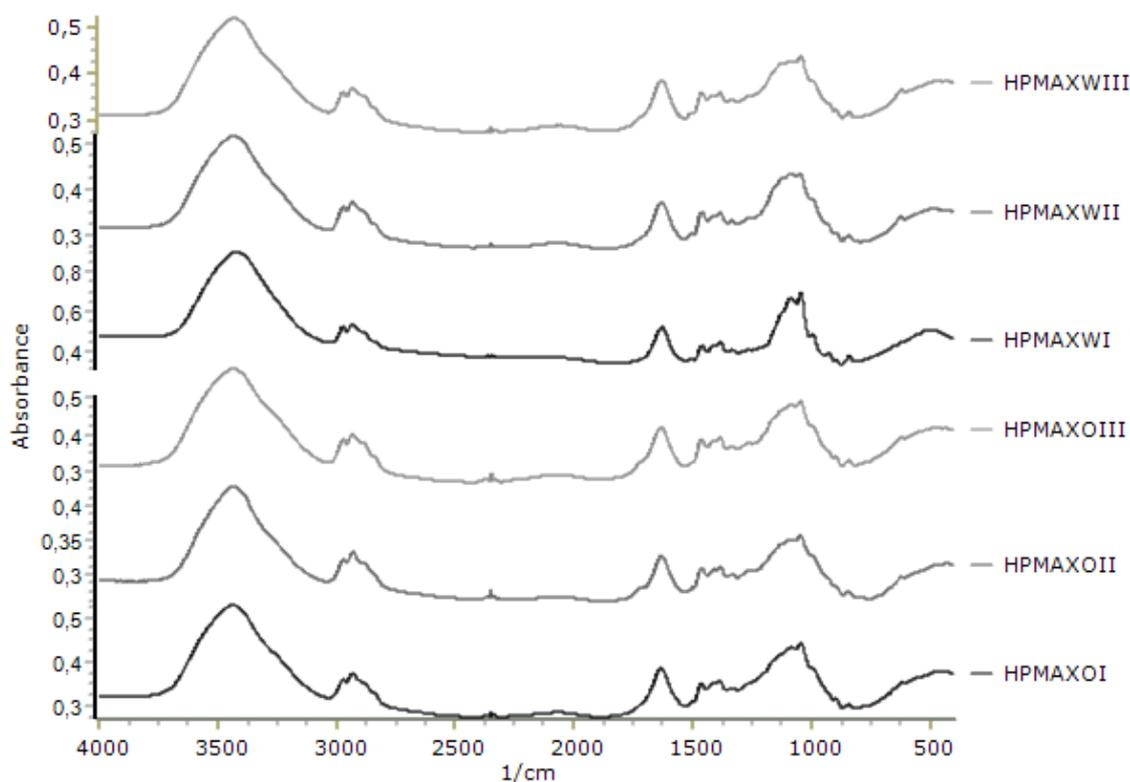
Figure 8. Spectrum of scaled up HPMAX from oat (HPMAXOI-HPMAXOIII) and wheat (HPMAXWI-HPMAXWIII).
