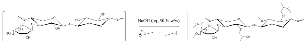
Figure 2. Schematic picture of how hydroxypropyl and methyl groups attach to the arabinoxylan chain.
