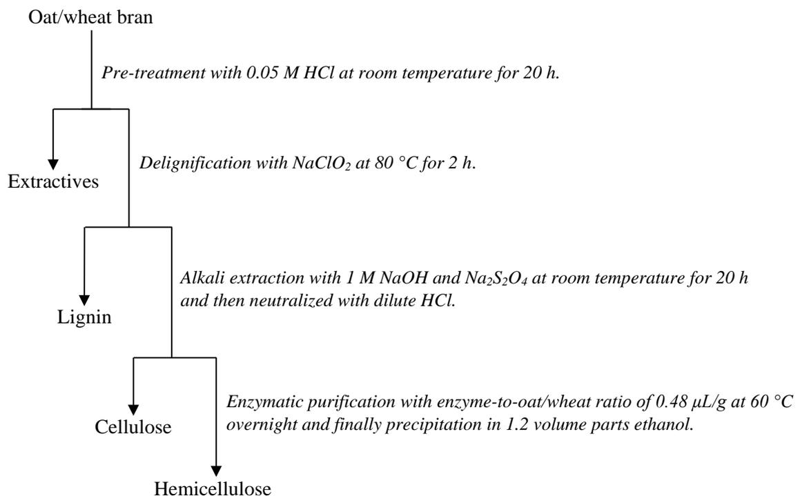
Figure 3. Schematic flow chart representing the extraction process of hemicellulose.
