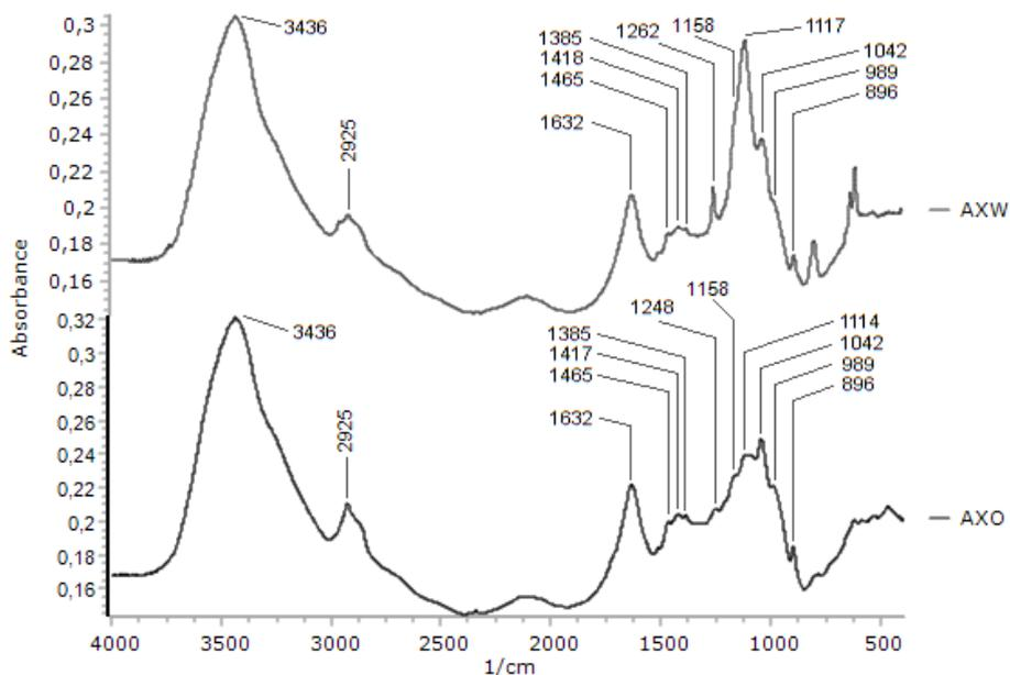
Figure 4. Spectrum of isolated arabinoxylan from oat (AXO) and wheat (AXW) in the infrared region of 4000-400  $\text{cm}^{-1}$ . The peaks highlighted show signs of chemical group as well as typical signs of arabinoxylan.
