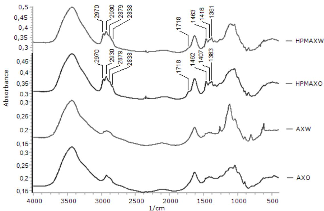
Figure 6. Spectrum of isolated arabinoxylan from oat (AXO), wheat (AXW) and their respective hydroxypropyl derivatives (HPMAXO and HPMAXW) in the infrared region of 4000-400  $\text{cm}^{-1}$ . The peaks highlighted show typical signs of conjugated hydroxypropyl groups.
