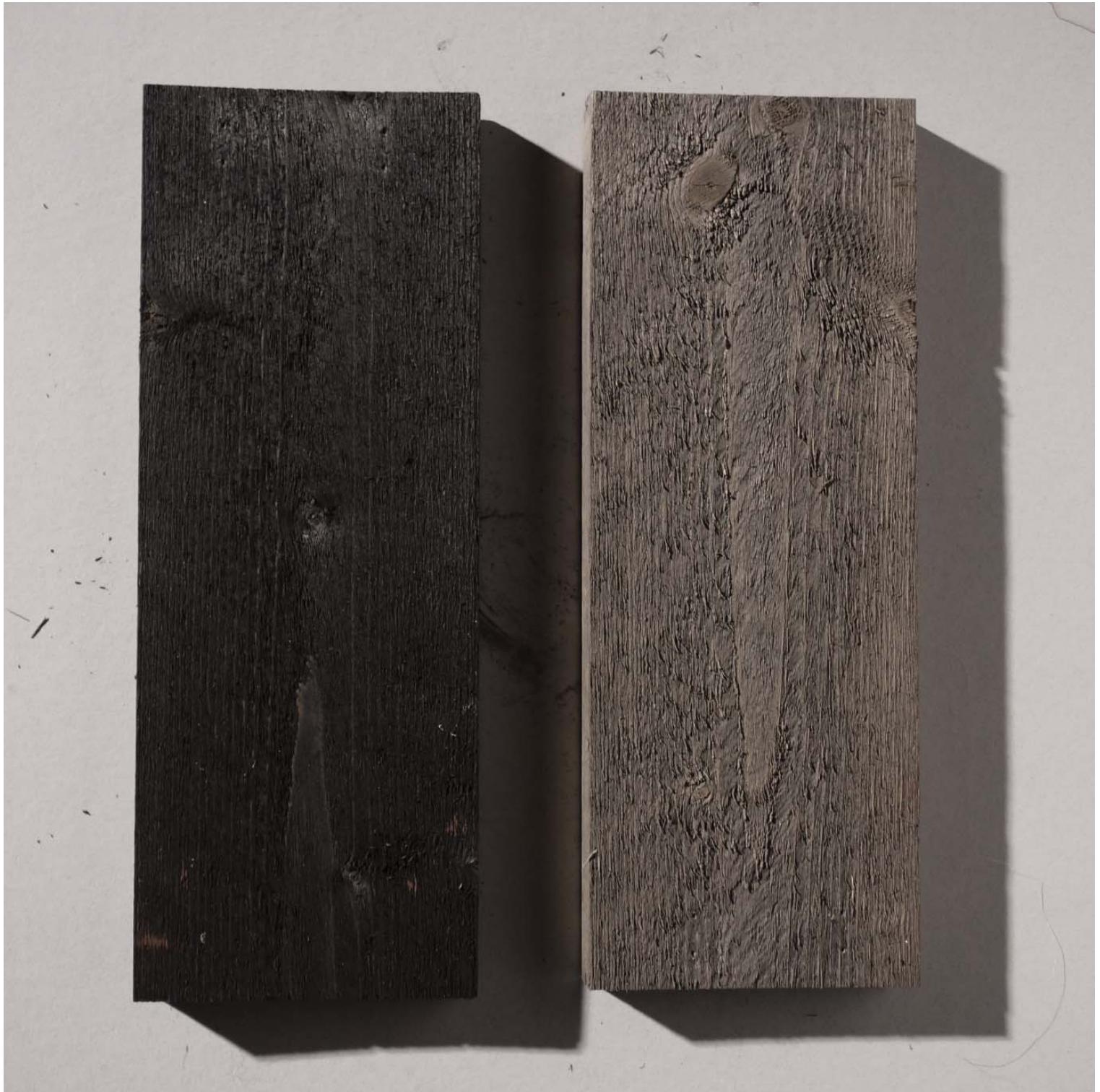
Material study, "tjärvitriol" an combination of copperas and tar. Dark inside to catch the reflections of the lake.
