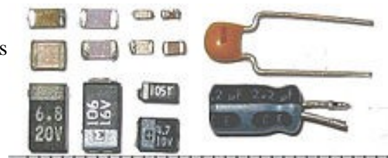
Illustration 4: Left side displays different sizes of surface mount capacitors. Top right side is a tantalum through-hole capacitor, and at the bottom right side is a electrolytic through-hole capacitor
