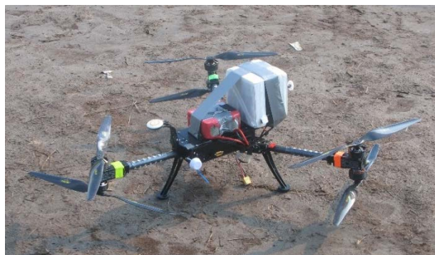
Figure 1. –left– Charge consumption measured with the SkyEye Micro drone in a high-altitude test with a payload similar to the gas sensor for volcanic plumes. –right– The Micro+Sunkist system ready to take-off at Bagana. The Sunkist is inside a fabrics box with the inlet pointing in direction of the drone's nose. The Li-ion battery pack is behind the Sunkist. The total payload should be placed to keep the centre of mass equidistant to the rotor pairs. Behind the batteries the GPS and communication antennas are shown, as well as the power connector (unplugged) behind the batteries
