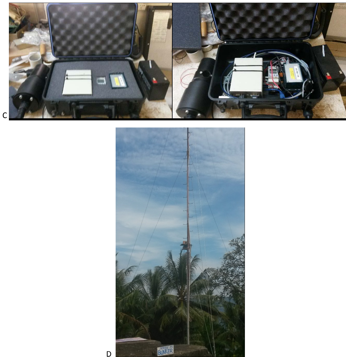
Figure 3b. (C) Instrument in the lab. (D) Instrument installed in the mast of the RVO Matupit station, viewed from north. The scanner is mounted on a platform which also offers shadow to the Peli box containing the instruments. Data and power cables are connected to the existing radio/power installations inside the Japanese Bunker
