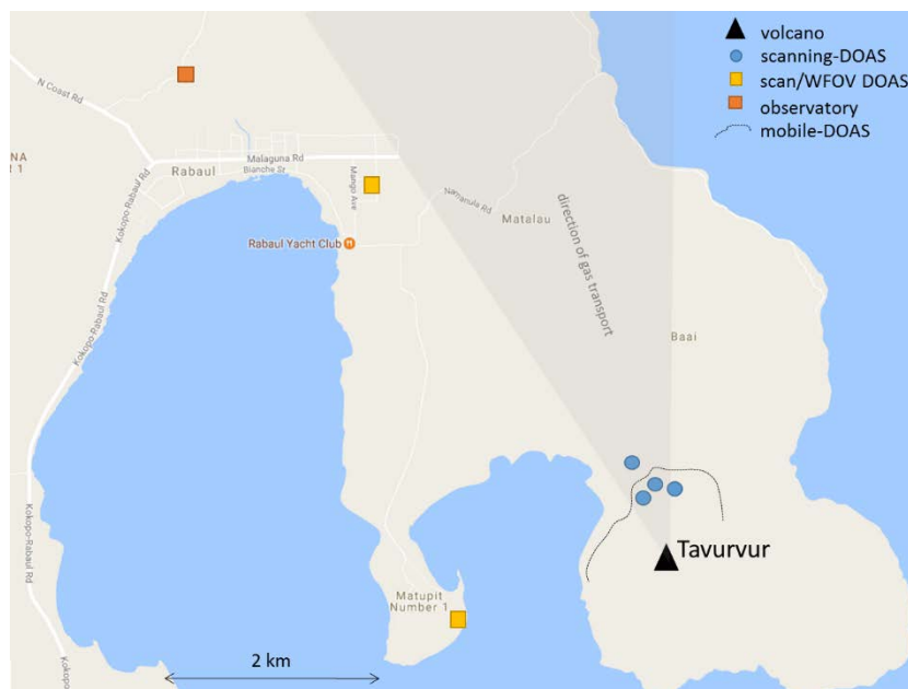
Figure 4. Map showing the locations of instruments used for measurements of the SO 2 flux from Tavurvur. Campaign measurements include temporary deployment of scanning-DOAS (blue circles) and mobile-DOAS traverses (dotted line). Long-term measurements included scanning-DOAS (since 2015) and a WFOV-DOAS instrument installed during the campaign. Data from the stations is transmitted to RVO
