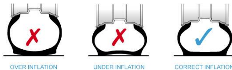
Figure 19 – The inflation pressure will affect the footprint (Tyrecity, 2017)
