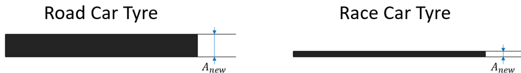
Figure 24 – The depth of a new tyre is different for road and race cars
