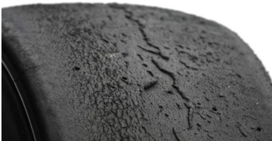
Figure 38 – During graining, tyre pieces are being rolled and torn off the tyre
