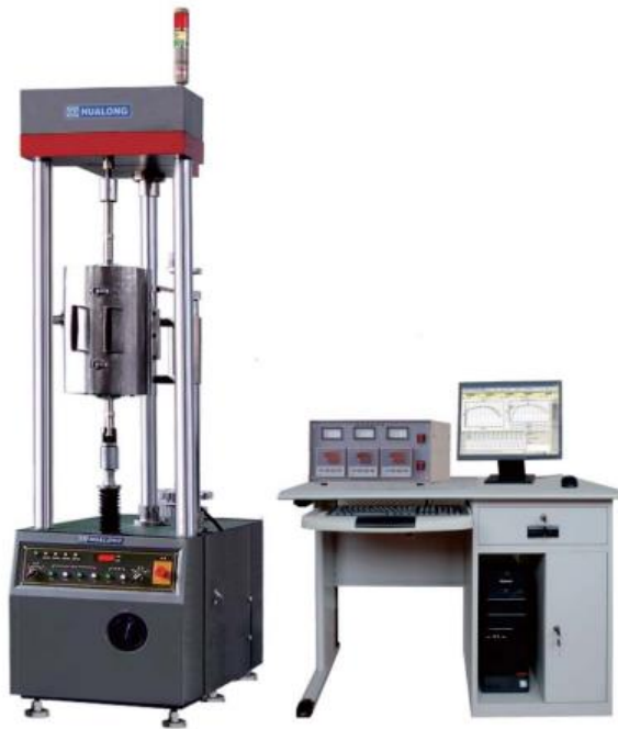
Figure 2.3 Hualong stress rupture testing machine - RCW series.
