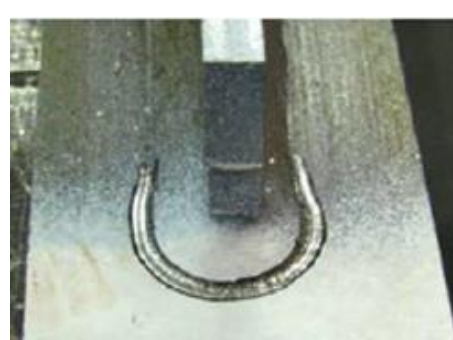
Figure 4.3 Weld toe profile before and after HFMI treatment, from Marquis and Barsoum (2016).
