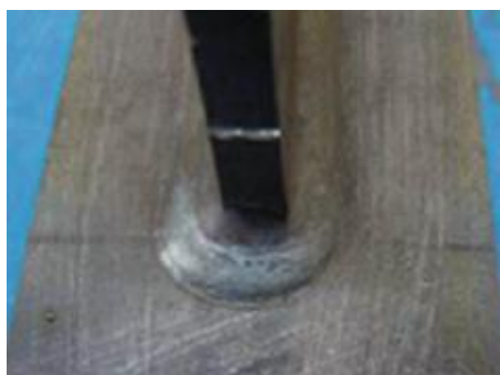
Figure 4.3 Weld toe profile before and after HFMI treatment, from Marquis and Barsoum (2016).
