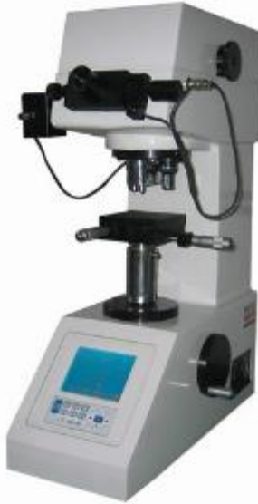
Figure 2.8 Jinan precision testing equipment Vickers hardness tester, 200HVS-5 model.
