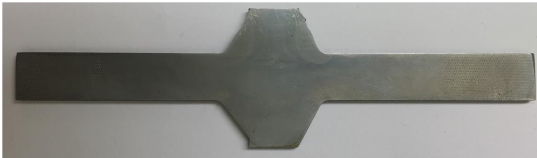
Figure 6.7 Polished test specimen for static testing.
