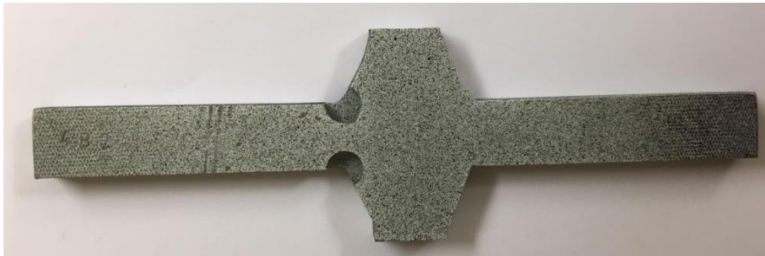
Figure 6.10 Painted test specimen for cyclic testing.
