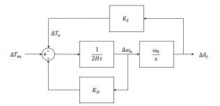
Fig. 3.4: Block diagram of the model of the SMIB-system considered in the first objective.
