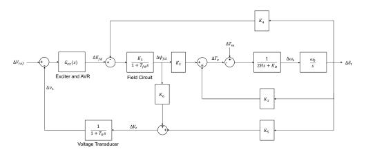
Fig. 3.6: Block diagram of the model of the SMIB-system also including the excitation system.
