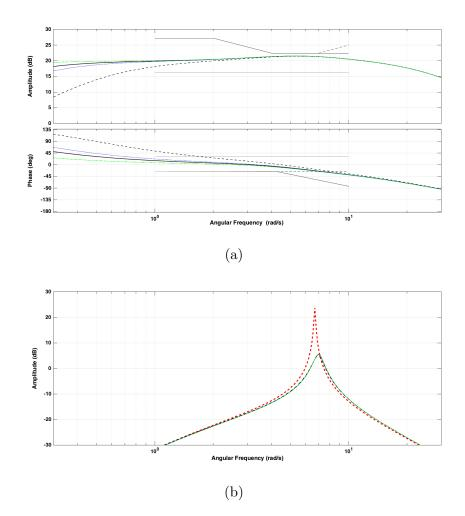
**Fig. 5.9:** Varying  $T_{W1}$  and  $T_{W2}$ . Solid:  $T_{W1} = T_{W2} = 7$  s; dashed:  $T_{W1} = T_{W2} = 2$  s; blue dotted:  $T_{W1} = T_{W2} = 5$  s; and green dash-dotted:  $T_{W1} = T_{W2} = 14$  s. (a) FIKS-method. (b) NG-method. Red dashed: PSS disconnected.
