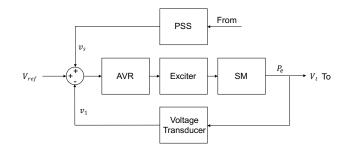
Fig. 2.16: Measurement points of the first evaluation method.
