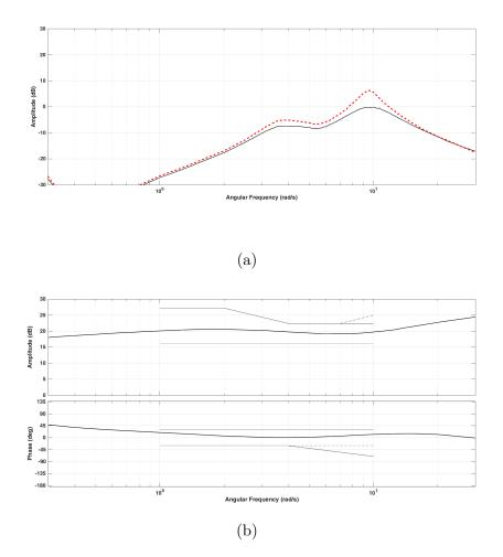
**Fig. 6.12:** PSS2B at bus 4062 is tuned according to the NG-method with tuning A. (a) NG-method. Solid: PSS connected and red dashed: PSS disconnected. (b) FIKS-method.
