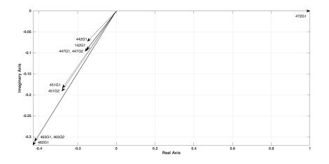
Fig. 4.6: Mode shape of the oscillation mode associated with the complex eigenvalue O5.
