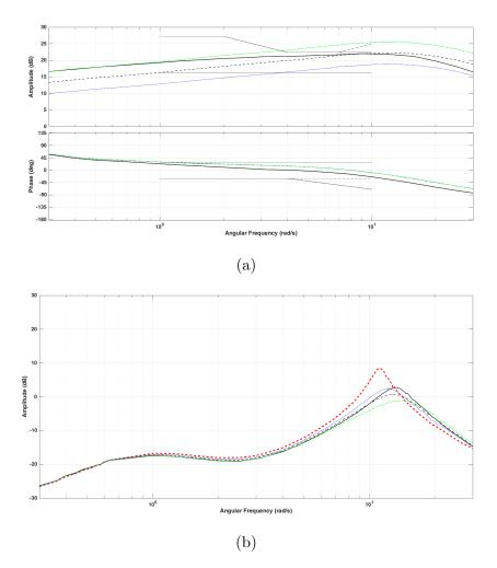
**Fig. 6.5:** New phase characteristics of the FIKS-method are above the reference phase characteristic. Solid: reference response; dashed: medium amplitude characteristic; blue dotted: low amplitude characteristic; and green dash-dotted: high amplitude characteristic. (a) FIKS-method. (b) NG-method. Red dashed: PSS disconnected.
