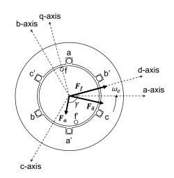
Fig. 2.2: The field MMF-wave  $(F_f)$  and the armature reaction MMF-wave  $(F_a)$  forms the resultant air-gap MMF-wave  $(F_{\delta})$ .
