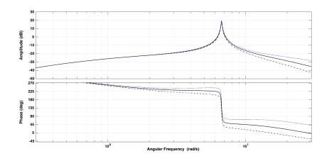
Fig. 5.11: Open-loop response from the voltage reference deviation to the PSS output for different values of r. Solid:  $r_0 = 2.941$ ; dashed: r = 2; and blue dotted: r = 5.
