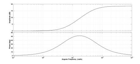
Fig. 2.12: Response of the lead-lag filter with  $T_{ll1} = 0.17$  s and  $T_{ll2} = 0.02$  s.
