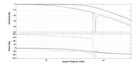
Fig. 5.1: Response from the PSS output to the terminal voltage deviation for different operating conditions of the SM. Solid: offline, dashed: loaded, and dotted: lightly loaded.
