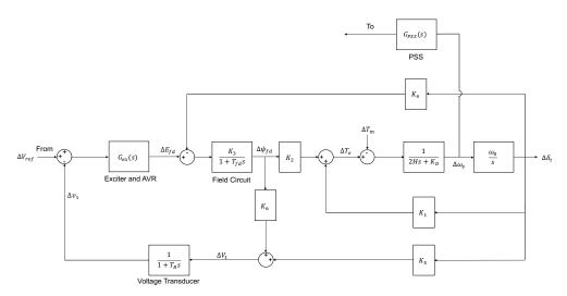
Fig. 5.7: Input and output points utilized to obtain the open-loop response from the voltage reference deviation to the PSS output.
