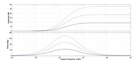
Fig. 2.14: Response of the lead-lag filter with varying filter order. Solid: N = 1, dashed: N = 2, and blue dotted: N = 3.
