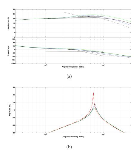
**Fig. 5.16:** Varying  $r_3$  while keeping  $r_1 = 2.941$  and  $r_2 = 2.941$ . Solid:  $r_0 = 2.941$ ; dashed:  $r_3 = 2$ ; blue dotted:  $r_3 = 2.941$ ; and green dash-dotted:  $r_3 = 5$ . (a) FIKS-method. (b) NG-method. Red dashed: PSS disconnected.
