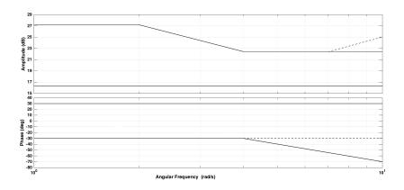
Fig. 2.17: Amplitude and phase limits of the FIKS-method. Solid: present limits and dashed: proposed limits.
