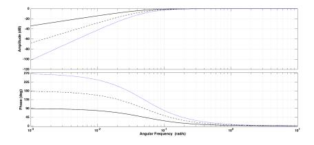
Fig. 2.11: Response of the washout filter with varying filter order. Solid: N = 1, dashed: N = 2, and blue dotted: N = 3.
