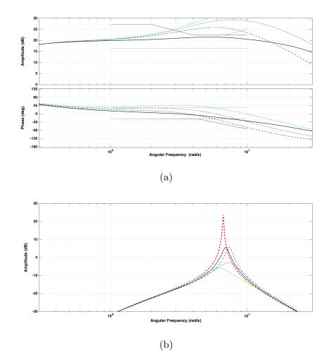
**Fig. 5.12:** Varying *r* after the initial halving of the break angular frequencies of  $G_{ll1}(s)$ ,  $G_{ll2}(s)$ , and  $G_{ll3}(s)$ . Solid:  $r_0 = 2.941$ ; dashed: r = 2; blue dotted: r = 2.941; and green dash-dotted: r = 5. (a) FIKS-method. (b) NG-method. Red dashed: PSS disconnected.
