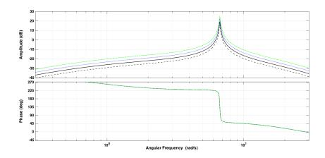
**Fig. 5.8:** Open-loop response from the voltage reference deviation to the PSS output for different values of  $K_{S1}$ . Solid:  $K_{S1} = 10$ ; dashed:  $K_{S1} = 7$ ; blue dotted:  $K_{S1} = 14$ ; and green dash-dotted:  $K_{S1} = 20$ .
