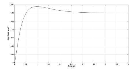
Fig. 4.3: Terminal voltage response when a 0.03 p.u. voltage reference step is applied at t = 0 s.
