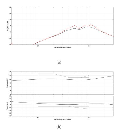
**Fig. 6.8:** PSS2Bs at bus 4063 are tuned according to the NG-method with tuning A. (a) NG-method. Solid: PSS connected and red dashed: PSS disconnected. (b) FIKS-method.
