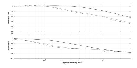
Fig. 6.1: Response from the PSS output to the terminal voltage for different operating conditions of the SM. Solid: offline, dashed: loaded, and dotted: lightly loaded.
