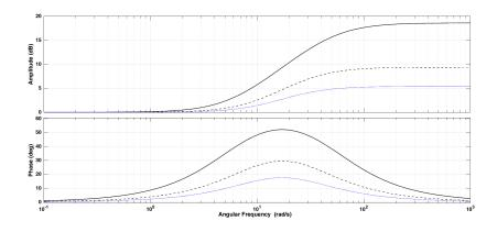
Fig. 2.13: Response of the lead-lag filter with varying ratio of  $T_{ll1}$  to  $T_{ll2}$ . Solid:  $T_{ll1}/T_{ll2} = 8.5$ ; dashed:  $T_{ll1}/T_{ll2} = 2.94$ ; and blue dotted:  $T_{ll1}/T_{ll2} = 1.86$ .
