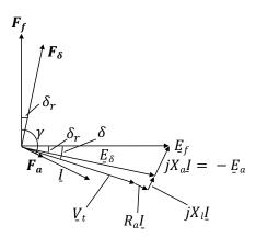
Fig. 2.4: Steady state phasor diagram of the SM.
