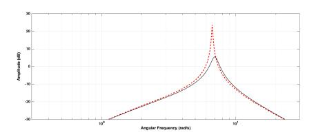
**Fig. 5.5:** Reference amplitude response obtained by the NG-method. Solid: PSS connected and red dashed: PSS disconnected.
