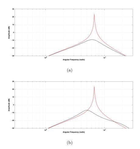
**Fig. 2.19:** Example responses obtained by the NG-method. Solid: PSS connected and red dashed: PSS disconnected. (a) Properly tuned PSS. (b) Improperly tuned PSS.
