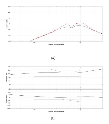
**Fig. 6.10:** PSS2Bs at bus 4063 are tuned according to the NG-method with tuning B. (a) NG-method. Solid: PSS connected and red dashed: PSS disconnected. (b) FIKS-method.
