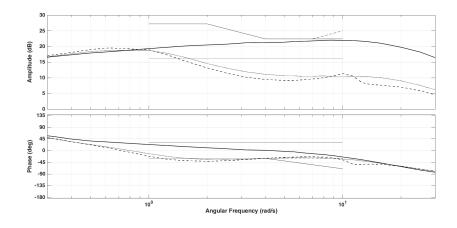
Fig. 6.2: Response obtained by the FIKS-method for different operating conditions of the SM. Solid: reference response (offline), dashed: loaded, and dotted: lightly loaded.
