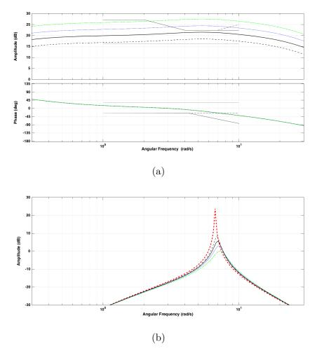
**Fig. 5.6:** Varying  $K_{S1}$ . Solid:  $K_{S1} = 10$ ; dashed:  $K_{S1} = 7$ ; blue dotted:  $K_{S1} = 14$ ; and green dash-dotted:  $K_{S1} = 20$ . (a) FIKS-method. (b) NG-method. Red dashed: PSS disconnected.
