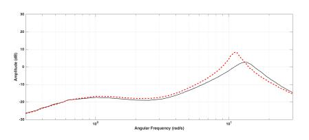
**Fig. 6.3:** Reference amplitude response obtained by the NG-method. Solid: PSS connected and red dashed: PSS disconnected.
