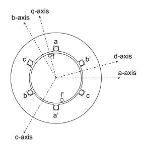
Fig. 2.1: Topology of a round-rotor SM.
