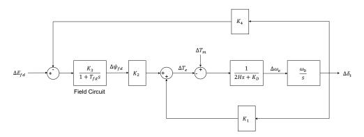
Fig. 3.5: Block diagram of the model of the SMIB-system also including the field circuit dynamics.
