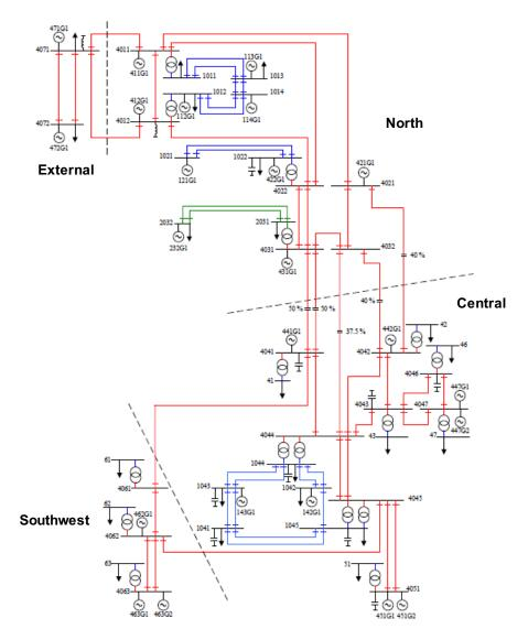
**Fig. 4.4:** Layout of the Nordic32-system. Red: 400 kV, green: 220 kV, and blue: 130 kV. (Published with courtesy of Joachim Andersson).
