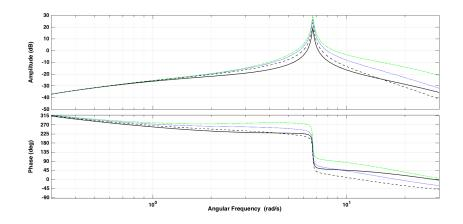
**Fig. 5.13:** Open-loop response from the voltage reference deviation to the PSS output for different values of r after the initial halving of the break angular frequencies of  $G_{ll1}(s)$ ,  $G_{ll2}(s)$ , and  $G_{ll3}(s)$ . Solid:  $r_0 = 2.941$ ; dashed: r = 2; blue dotted: r = 2.941; and green dash-dotted: r = 5.
