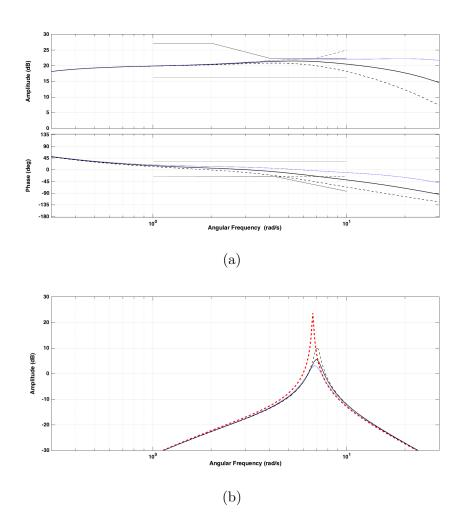
**Fig. 5.10:** Varying r. Solid:  $r_0 = 2.941$ ; dashed: r = 2; and blue dotted: r = 5. (a) FIKS-method. (b) NG-method. Red dashed: PSS disconnected.
