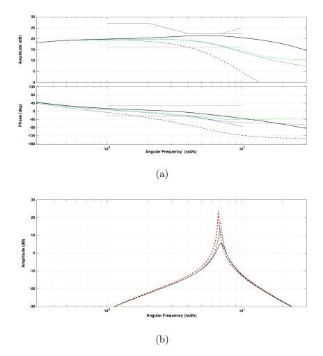
**Fig. 5.14:** Varying *r* after the initial doubling of the break angular frequencies of  $G_{ll1}(s)$ ,  $G_{ll2}(s)$ , and  $G_{ll3}(s)$ . Solid:  $r_0 = 2.941$ ; dashed: r = 2; blue dotted: r = 2.941; and green dash-dotted: r = 5. (a) FIKS-method. (b) NG-method. Red dashed: PSS disconnected.
