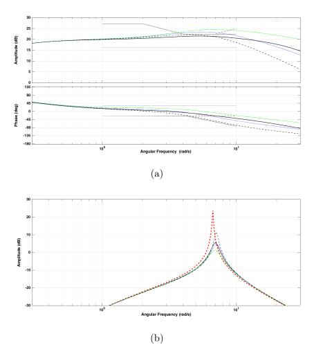
**Fig. 5.15:** Varying r after the break angular frequencies of  $G_{ll1}(s)$  and  $G_{ll3}(s)$  are initially doubled and halved, respectively. Solid:  $r_0 = 2.941$ ; dashed: r = 2; blue dotted: r = 2.941; and green dash-dotted: r = 5. (a) FIKS-method. (b) NG-method. Red dashed: PSS disconnected.
