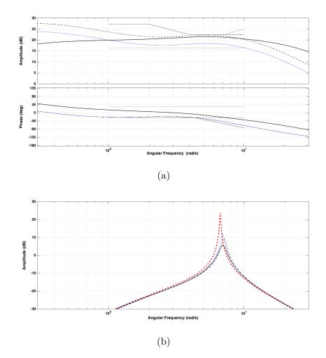
Fig. 5.17: New phase characteristics of the FIKS-method are below the reference phase characteristic. Solid: reference response; dashed: high amplitude characteristic; and blue dotted: low amplitude characteristic. (a) FIKS-method. (b) NG-method. Red dashed: PSS disconnected.
