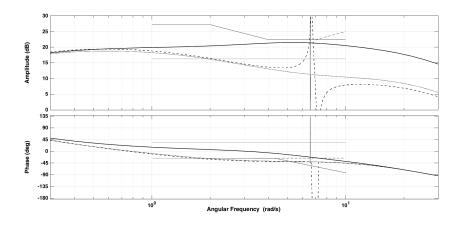
Fig. 5.3: Response obtained by the FIKS-method for different operating conditions of the SM. Solid: reference response (offline), dashed: loaded, and dotted: lightly loaded.
