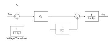
Fig. 4.2: Block diagram of the excitation system.
