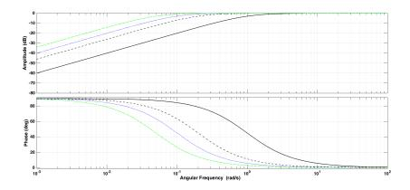
Fig. 2.10: Response of the washout filter with varying time constant. Solid:  $T_W = 1$  s, dashed:  $T_W = 5$  s, blue dotted:  $T_W = 10$  s, and green dash-dotted:  $T_W = 20$  s.
