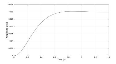
Fig. 3.8: Terminal voltage deviation response when a 0.03 p.u. step is applied to the voltage reference deviation at t = 0 s.
