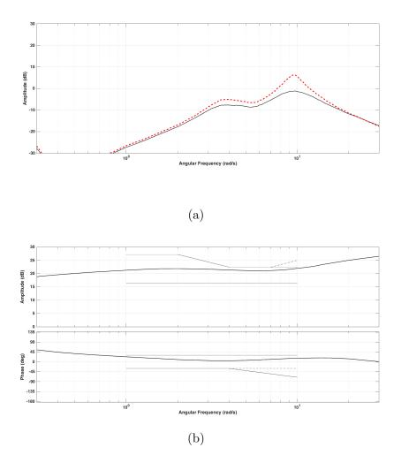
**Fig. 6.14:** PSS2B at bus 4062 is tuned according to the NG-method with tuning B. (a) NG-method. Solid: PSS connected and red dashed: PSS disconnected. (b) FIKS-method.
