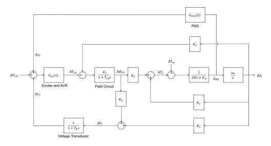
**Fig. 3.9:** Block diagram of the model of the SMIB-system also including the PSS.
