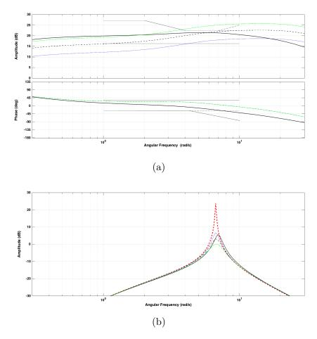
**Fig. 5.18:** New phase characteristics of the FIKS-method are above the reference phase characteristic. Solid: reference response; dashed: medium amplitude characteristic; blue dotted: low amplitude characteristic; and green dash-dotted: high amplitude characteristic. (a) FIKS-method. (b) NG-method. Red dashed: PSS disconnected.
