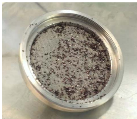
Figure 24 – Bilberry seeds on the top filter of the extraction vessel after formation of dry ice during depressurization of the reactor.
