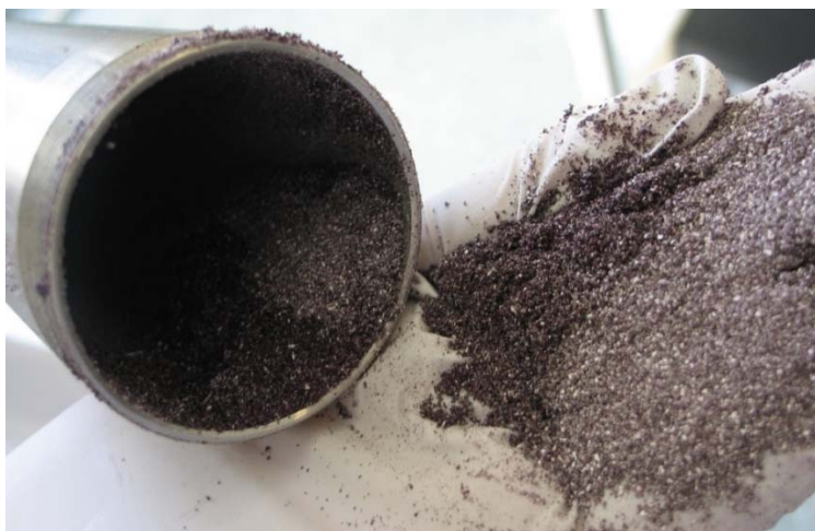
Figure 23 – Channeling in the extraction vessel, the darker material has not been exposed to CO 2 , while the light material has been properly extracted.
