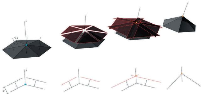
9 The developed Mesh Offset method for the FLB geometry.
