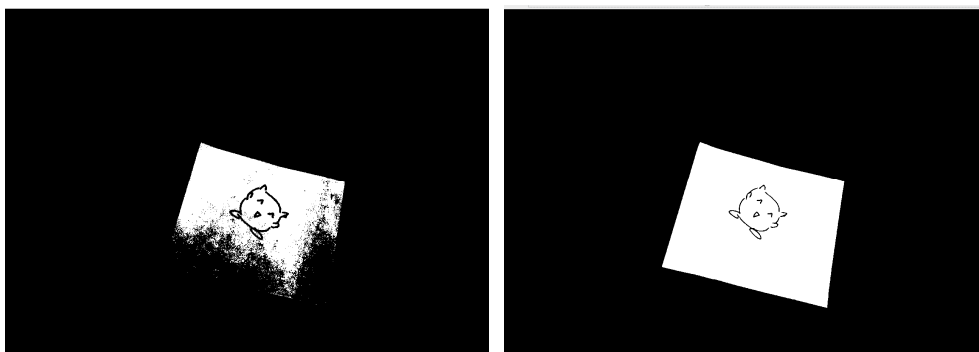
Figure 4.8 Resulting image after threshold in Figure 4.7, from left to right: Too high threshold, moderate threshold.
