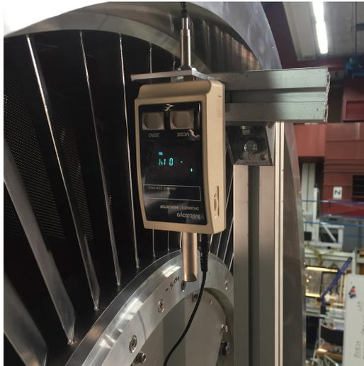
Figure A.4: *Clocking the LPT rotor shroud.*
