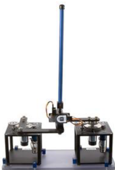
Figure 3.1: Experiment setup, Quanser 2 DOF Inverted Pendulum [15]
