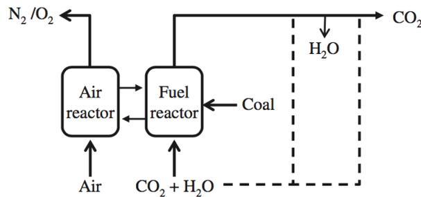
Figure 3.2: Schematic layout of a solid fuelled iG-CLC. Figure from [6]
