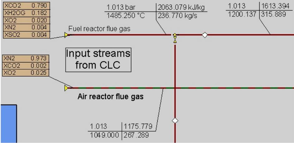
Figure 5.3: Flue gas input streams to the steam cycle
