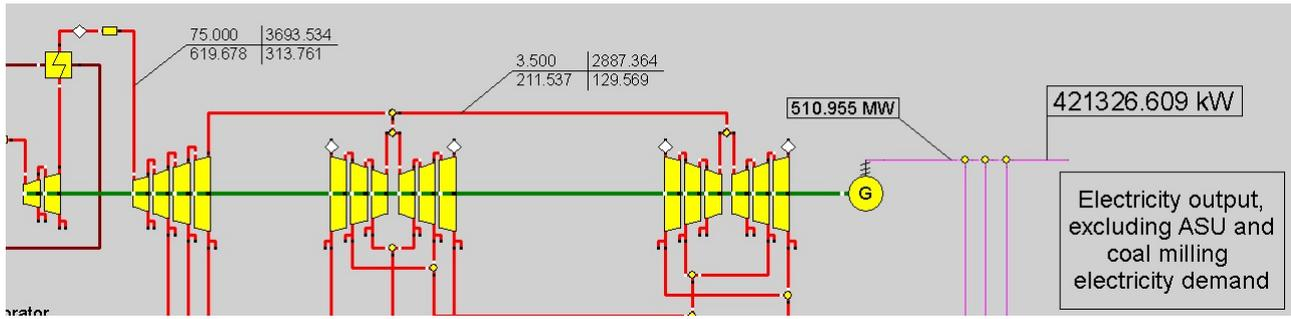
Figure 5.5: Steam turbine configuration
