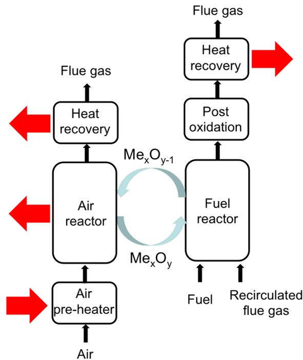
Figure 5.1: Heat transfer points between the steam cycle and the main CLC plant model
