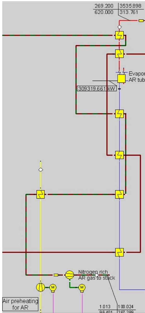
Figure 5.4: Flue gas path. Brown: FR flue gas stream, Brown/green: AR flue gas stream, Yellow: Air feed to the AR
