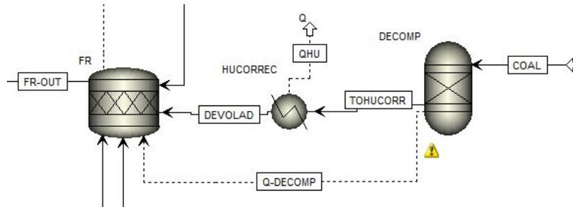
Figure 5.2: Pyrolysis of coal in the Aspen model
