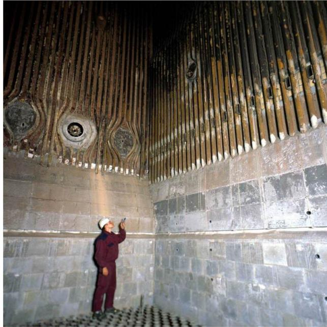
Figure 3.3: Bubbling fluidized bed reactor with walls covered by evaporator tubes. Figure from Teir, S. [16]
