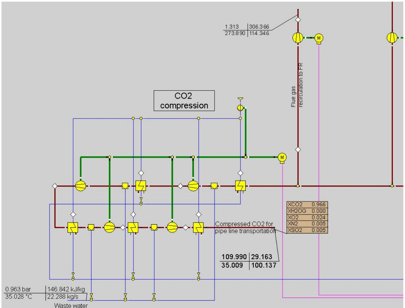
Figure 5.7: CO<sub>2</sub>-compression section
