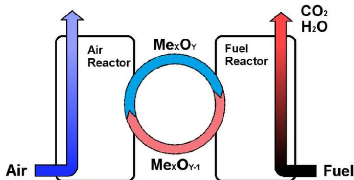
Figure 1.1: Illustration of a CLC interconnected fluidized-bed reactor system. Figure from Gunnarson, A. [48]
