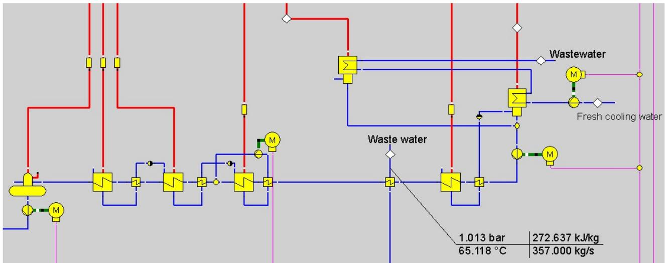
Figure 5.6: Feed water pre-heating system
