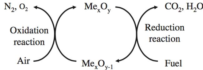
Figure 3.1: Chemical Looping Combustion system for gaseous fuels with a metal oxide as oxygen carrier. Figure from [6]
