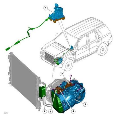
Figure 3.1: Location of the gearbox in a car [29].
