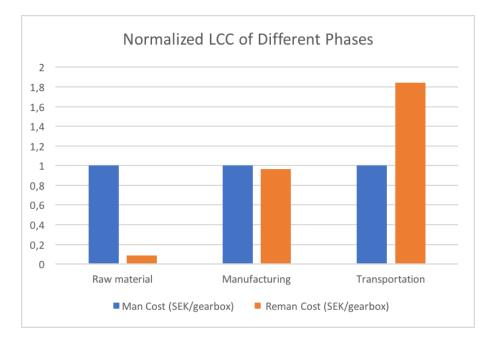
Figure 7.2: Normalized costs for manufactured and remanufactured gearbox
