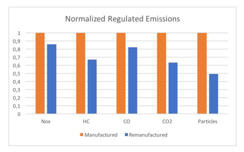
Figure 6.1: Normalized regulated emissions from manufactured and remanufactured gearbox over the whole life cycle.
