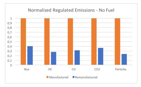
Figure 6.2: Normalized regulated emissions from manufactured and remanufactured gearbox, excluding the use phase, over the life cycle.
