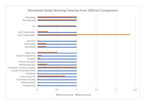
Figure 6.7: A comparison of contribution of each process or component towards Global Warming Potential, normalized with respect to a newly manufactured gearbox.
