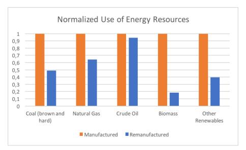
**Figure 6.4:** Use of different energy resources in manufactured and remanufactured gearbox over the whole life cycle.
