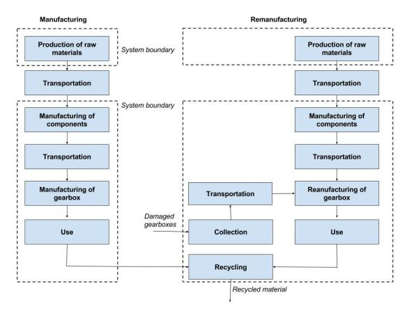
Figure 5.1: Initial flow chart showing the life cycle and natural boundaries of both new and remanufactured gearbox.
