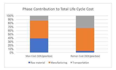
Figure 7.1: Comparison of costs for different phases, excluding the use phase, in manufactured and remanufactured gearbox
