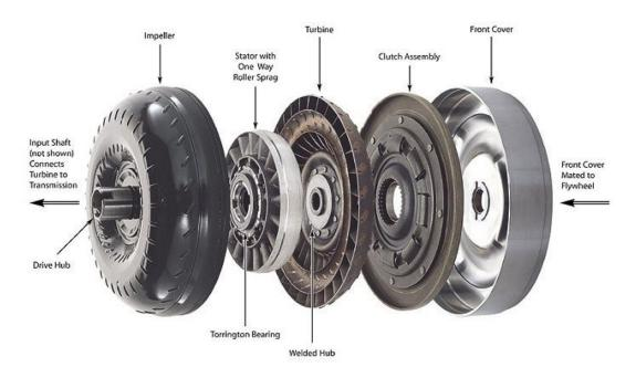
Figure 3.3: An exploded view of a torque converter [32].
