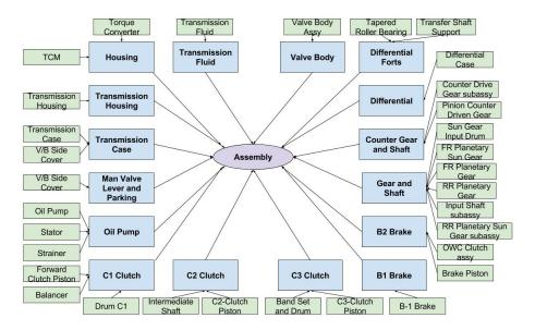
Figure 5.2: Gearbox Assembly Structure with sub-assembly processes and parts.
