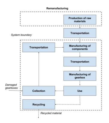
Figure 6.9: Flowchart for End Of Life collection with Remanufacturing Scenario Since collected parts are already modelled in the previous system, this will only
