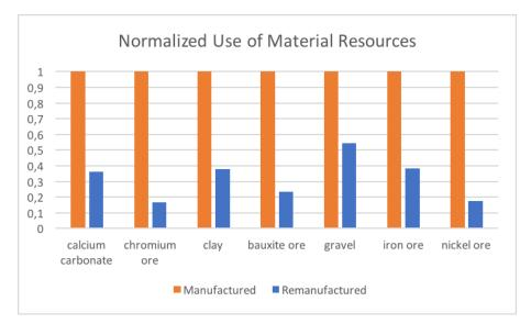
Figure 6.3: Normalized use of material resources in manufactured and remanufactured gearbox over the whole life cycle.
