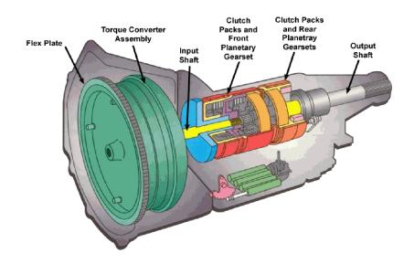
Figure 3.2: Various components in a gearbox [30].
