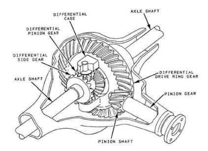
Figure 3.4: A cut open view of a differential [37].
