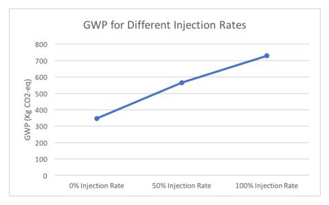
Figure 6.8: Effect on Global Warming Potential for different injection rates.
