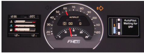
(a) Yellow flashing arrow and display indicating that a lane-change is ordered by human driver or utility function.
