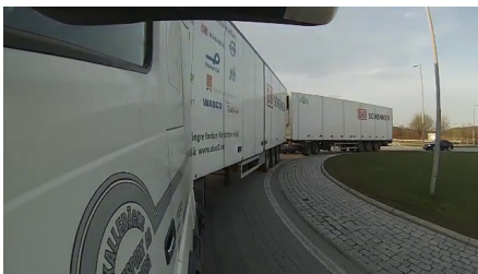
(a) Off-tracking in low speed roundabout driving using an A-double combination. (b) Rearward amplification in a severe lane change manoeuvre.
