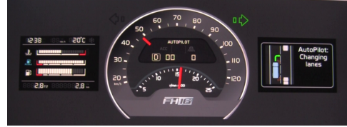
(b) Green flashing light and display indicating that lane change is started.
