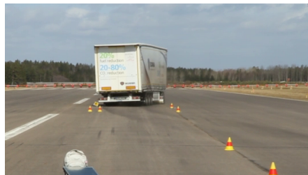
(a) Off-tracking in low speed roundabout driving using an A-double combination. (b) Rearward amplification in a severe lane change manoeuvre.
