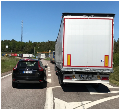
Figure 1.1: Difference in height and width between a passenger car and heavy truck combination. This affects the risk of roll-over and available lane space. The static roll-over limit for heavy trucks can be as low as 0.35g , whereas the roll-over limit for passenger cars is typically 1.1g .
