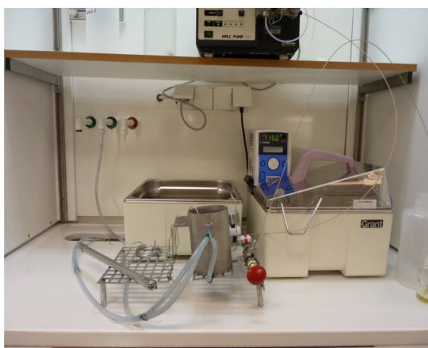
Figure 3.2. Image of the small-scale flow-through reactor used
