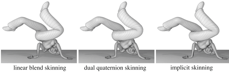
Fig. 6. Dana model in a break-dance pose. From left to right , the model is deformed with linear blend skinning, dual quaternion skinning and implicit skinning. Note the visible loss of volume produced by LBS ( left ). Implicit skinning ( right ), however, generates visually plausible skin deformations, which avoids the artefacts of linear blend skinning, as well as the bulging artefacts of dual quaternion skinning [83].
