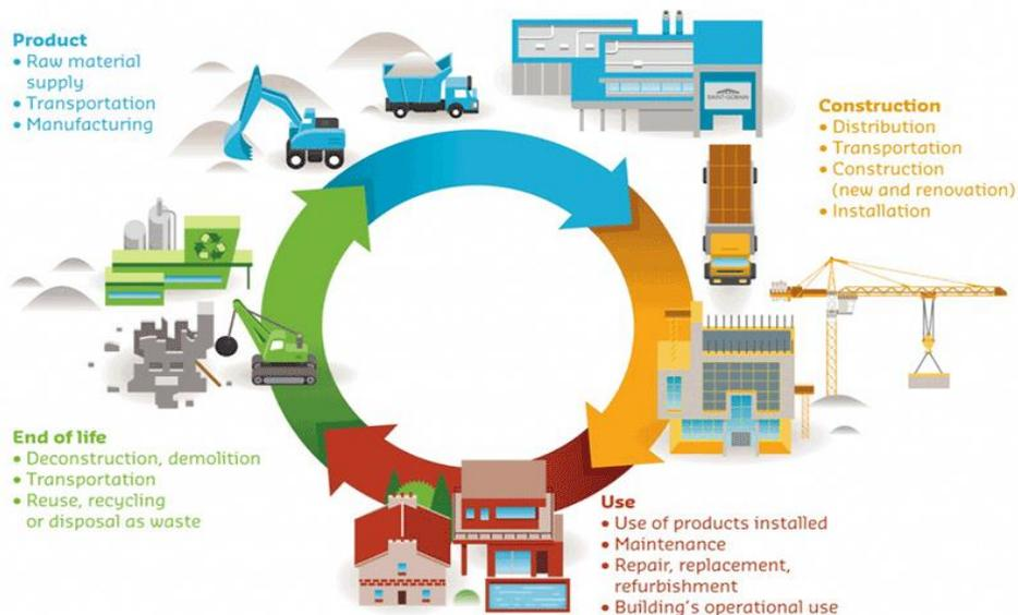
Figure 1. The life cycle of a construction product (Saint-Gobain, 2017).
